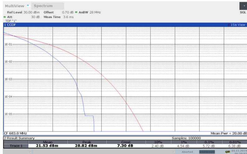
**LTE band 71 , 20MHz Bandwidth,16QAM**
