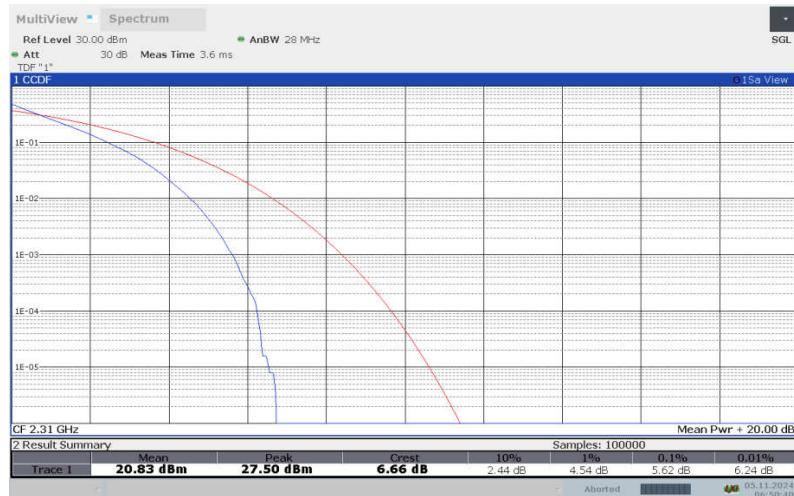
**LTE band 30 , 10MHz Bandwidth,16QAM**
