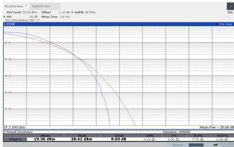
**LTE band 41 , 20MHz Bandwidth,16QAM**
