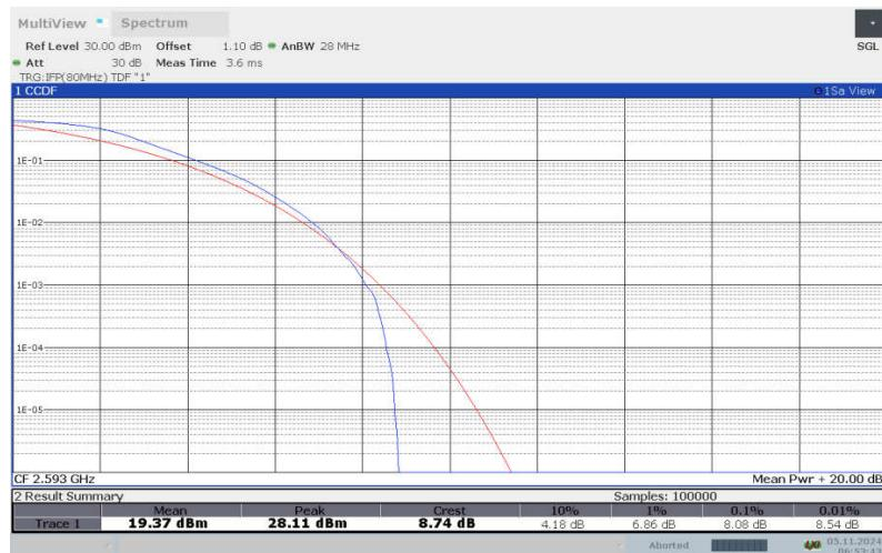
**LTE band 41 , 15MHz Bandwidth,16QAM**
