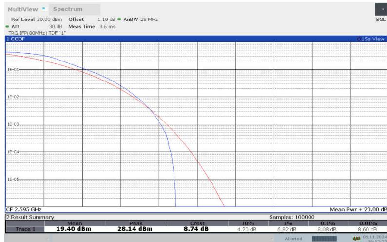
**LTE band 38 , 15MHz Bandwidth,16QAM**
