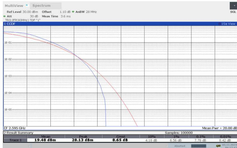
**LTE band 38 , 20MHz Bandwidth,16QAM**
