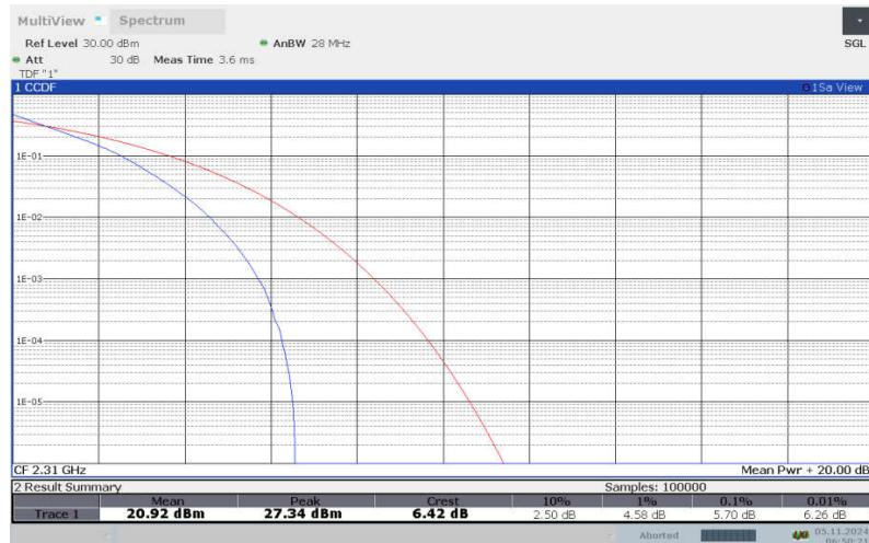
**LTE band 30 , 5MHz Bandwidth,16QAM**
