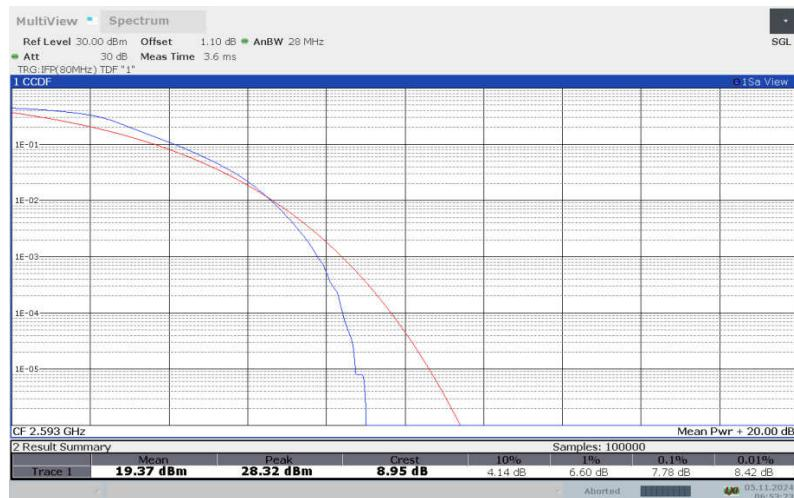
**LTE band 41 , 10MHz Bandwidth,16QAM**
