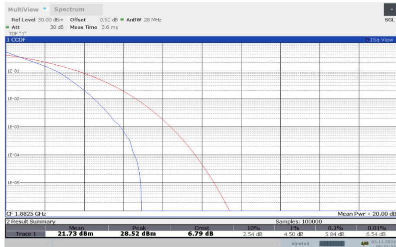
**LTE band 25 , 3MHz Bandwidth,16QAM**
