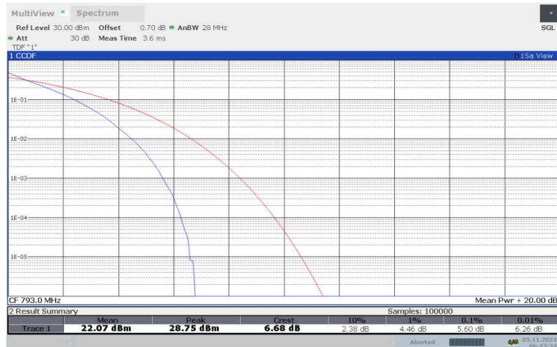
**LTE band 14 , 10MHz Bandwidth,16QAM**
