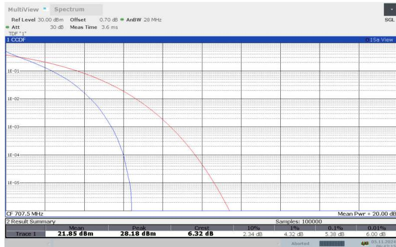
**LTE band 12 , 10MHz Bandwidth,16QAM**
