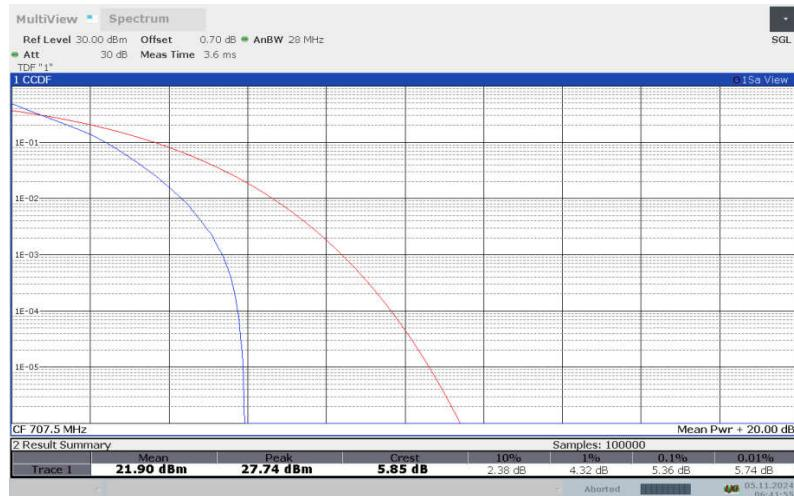
**LTE band 12 , 5MHz Bandwidth,16QAM**
