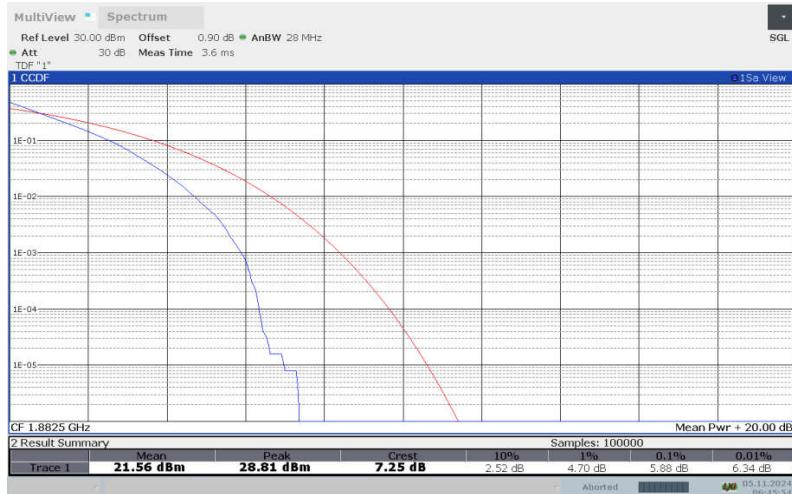
**LTE band 25 , 15MHz Bandwidth,16QAM**
