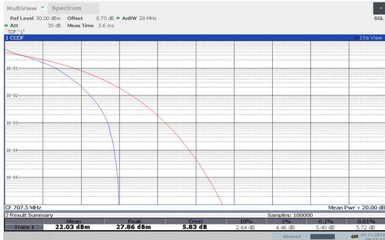
**LTE band 12 , 1.4MHz Bandwidth,16QAM**
