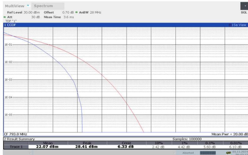
**LTE band 14 , 5MHz Bandwidth,16QAM**
