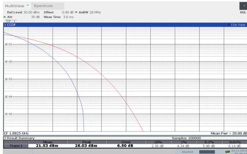
**LTE band 25 , 20MHz Bandwidth,16QAM**
