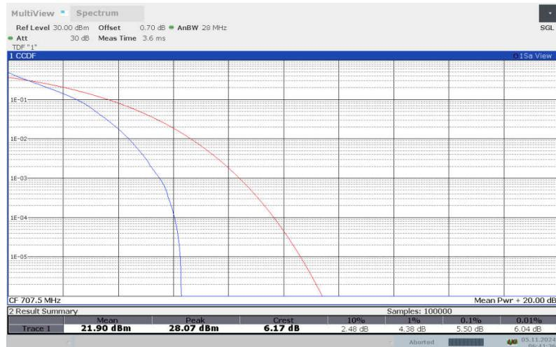
**LTE band 12 , 3MHz Bandwidth,16QAM**
