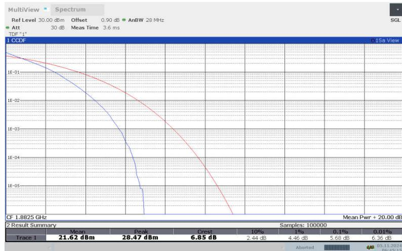
**LTE band 25 , 5MHz Bandwidth,16QAM**
