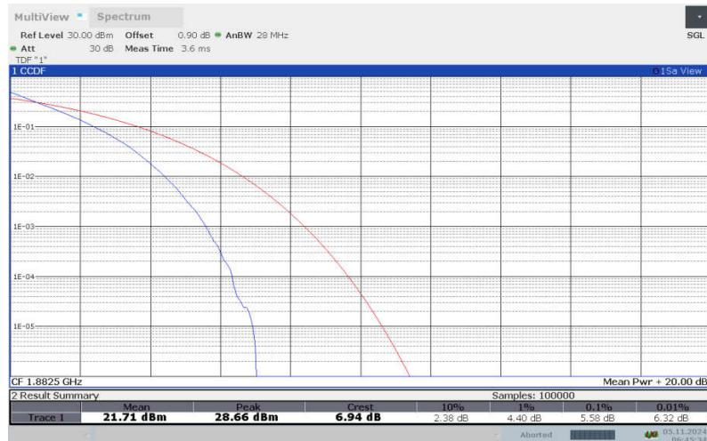
**LTE band 25 , 10MHz Bandwidth,16QAM**
