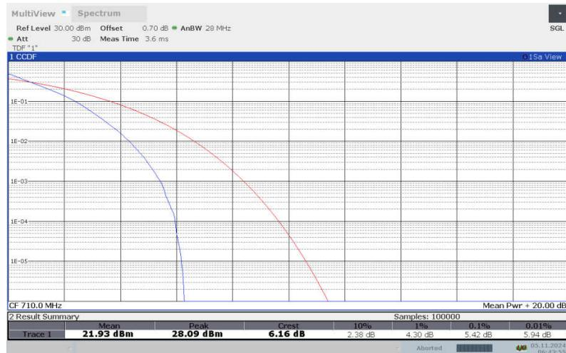
**LTE band 17 , 5MHz Bandwidth,16QAM**
