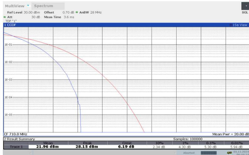
**LTE band 17 , 10MHz Bandwidth,16QAM**
