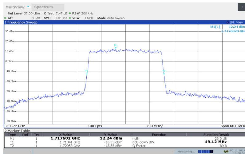
**LTE band 66 , 20MHz Bandwidth, LOW, 64QAM (-26dBc BW)**
