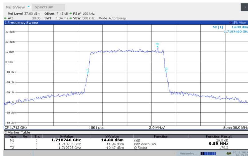
**LTE band 66 , 10MHz Bandwidth, LOW, 64QAM (-26dBc BW)**
