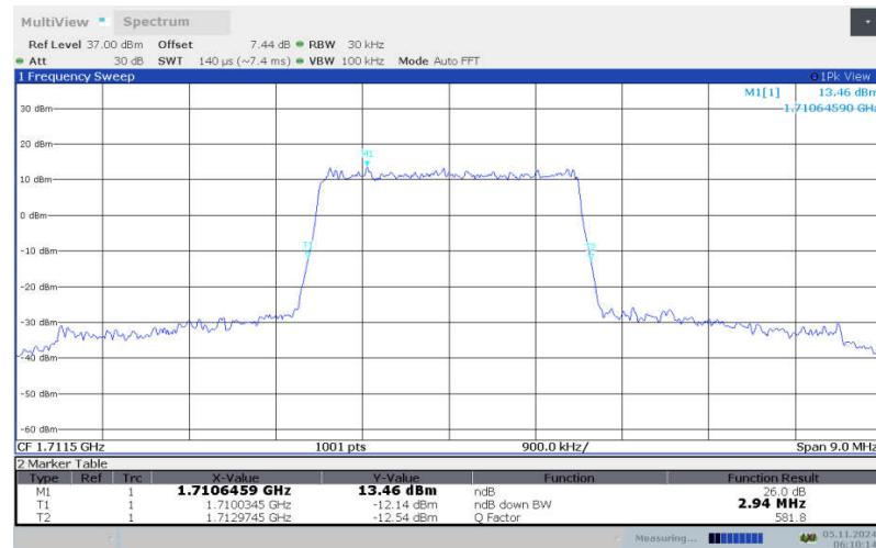
**LTE band 66 , 3MHz Bandwidth, LOW, 16QAM (-26dBc BW)**
