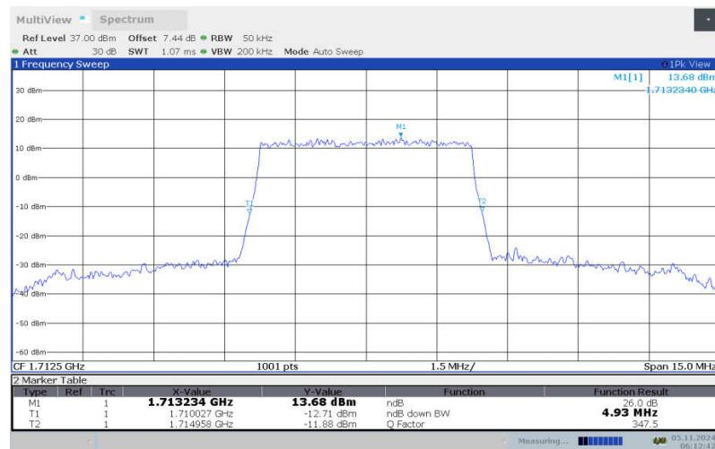
**LTE band 66 , 5MHz Bandwidth, LOW, 16QAM (-26dBc BW)**
