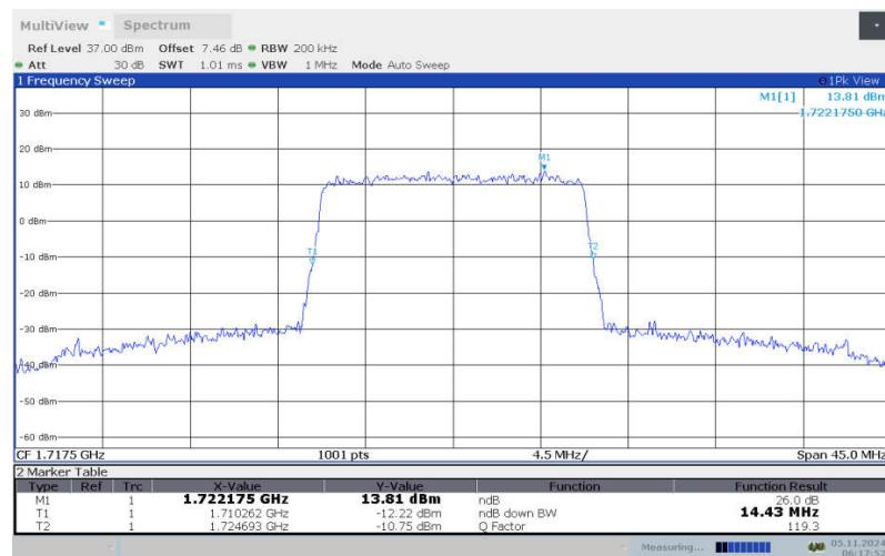
**LTE band 66 , 15MHz Bandwidth, LOW, 64QAM (-26dBc BW)**
