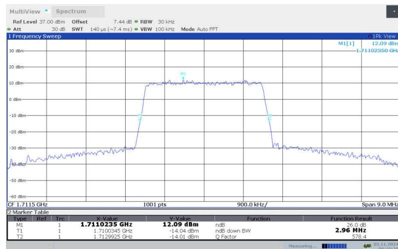
**LTE band 66 , 3MHz Bandwidth, LOW, 64QAM (-26dBc BW)**
