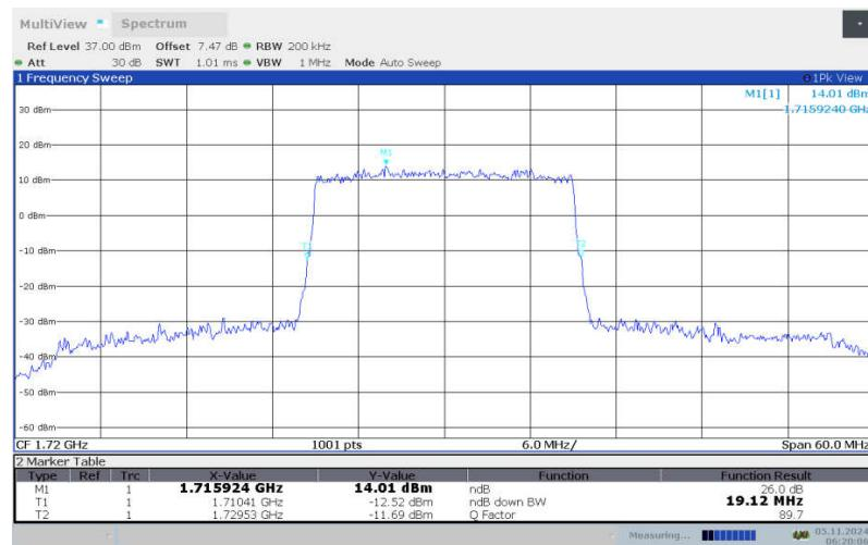
**LTE band 66 , 20MHz Bandwidth, LOW, 16QAM (-26dBc BW)**
