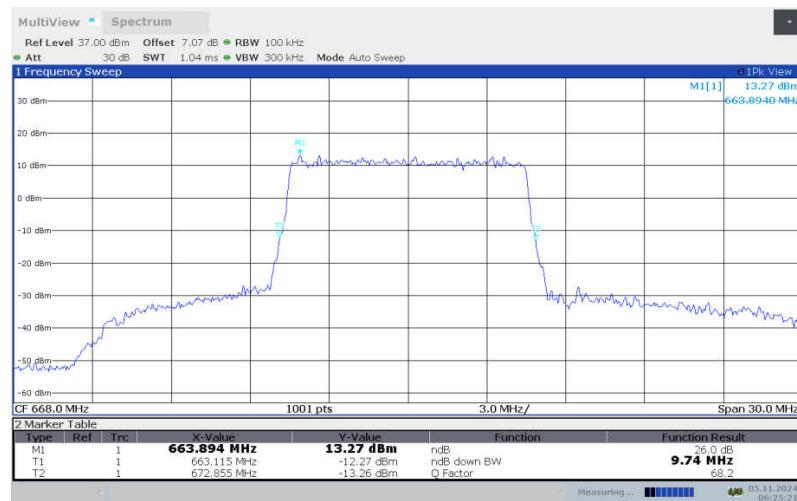
**LTE band 71 , 10MHz Bandwidth, LOW, 16QAM (-26dBc BW)**
