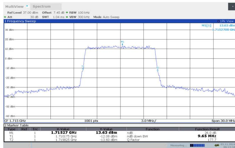
**LTE band 66 , 10MHz Bandwidth, LOW, 16QAM (-26dBc BW)**
