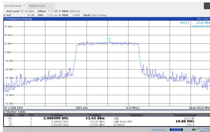
**LTE band 41 , 20MHz Bandwidth, LOW, 16QAM (-26dBc BW)**
