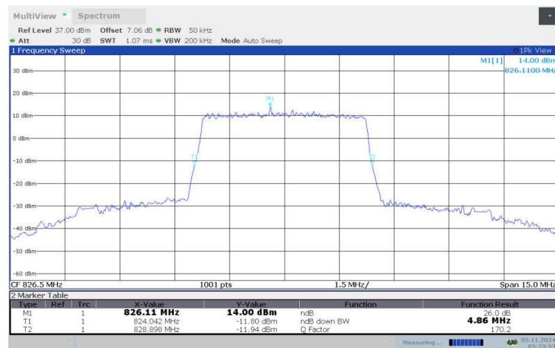
**LTE band 26 , 5MHz Bandwidth, LOW, 64QAM (-26dBc BW)**
