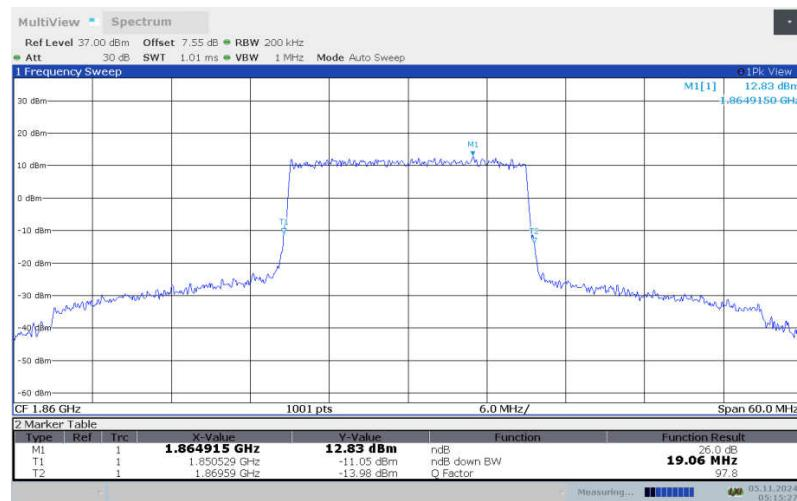
**LTE band 25 , 20MHz Bandwidth, LOW, 16QAM (-26dBc BW)**
