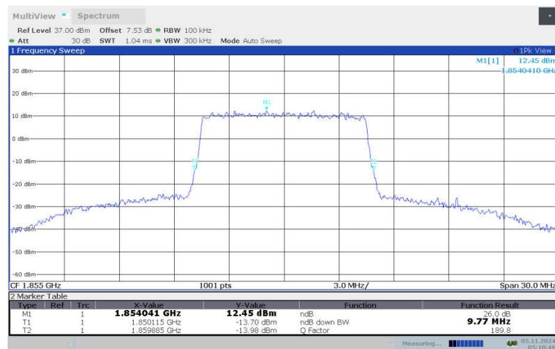
**LTE band 25 , 10MHz Bandwidth, LOW, 64QAM (-26dBc BW)**
