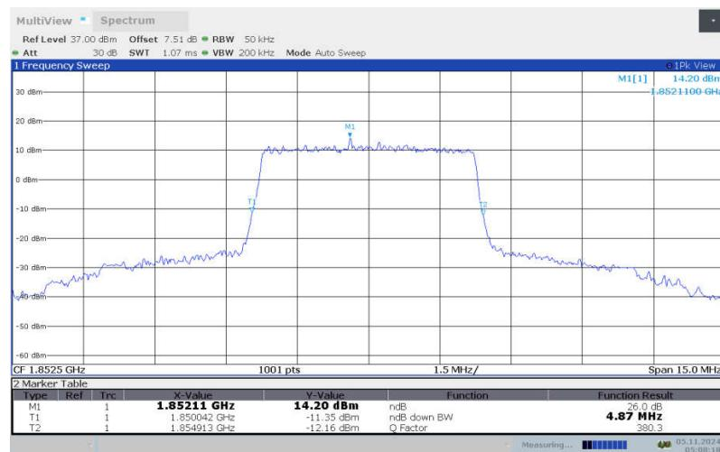
**LTE band 25 , 5MHz Bandwidth, LOW, 64QAM (-26dBc BW)**
