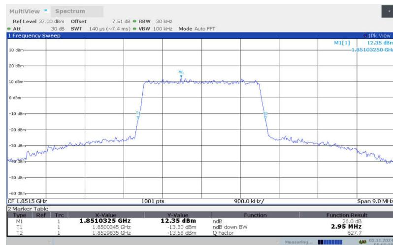
**LTE band 25 , 3MHz Bandwidth, LOW, 64QAM (-26dBc BW)**
