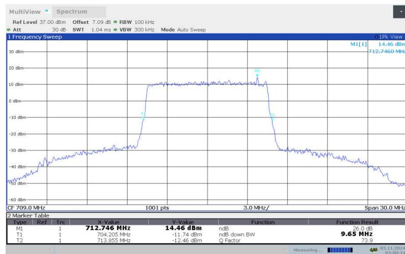
**LTE band 17 , 10MHz Bandwidth, LOW, 64QAM (-26dBc BW)**
