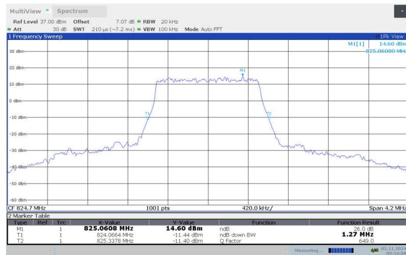
**LTE band 26 , 1.4MHz Bandwidth, LOW, 16QAM (-26dBc BW)**
