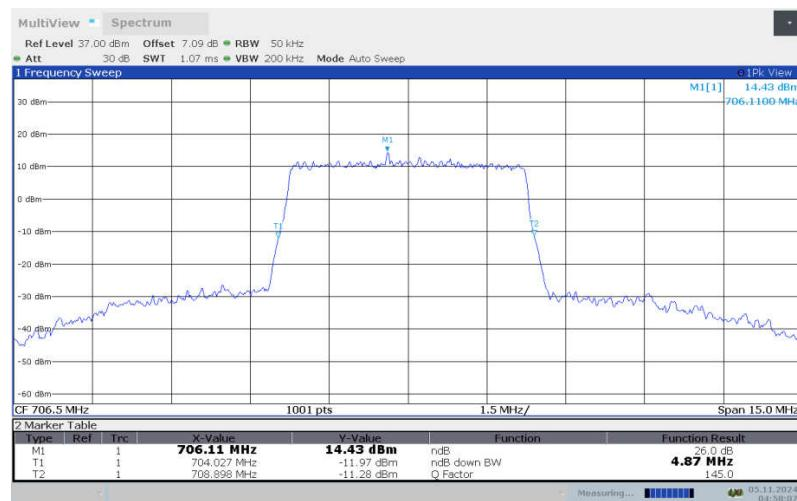
**LTE band 17 , 5MHz Bandwidth, LOW, 64QAM (-26dBc BW)**
