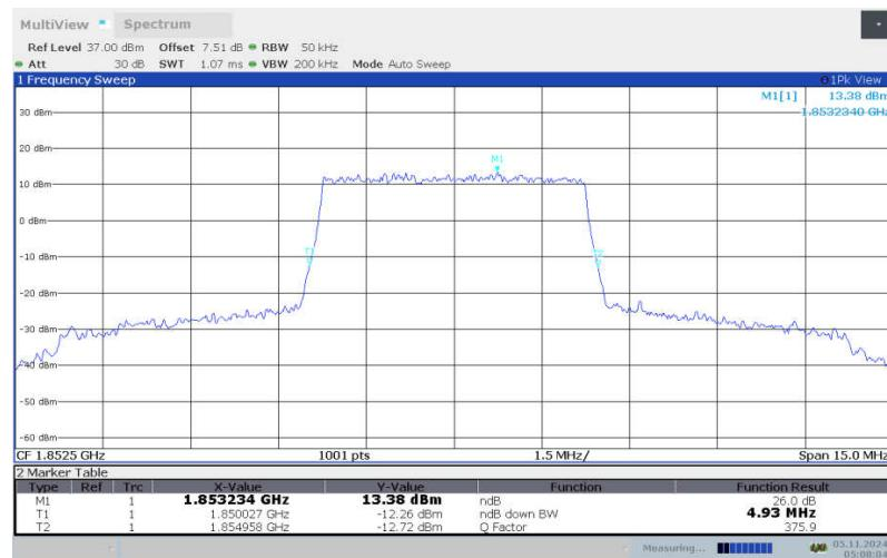
**LTE band 25 , 5MHz Bandwidth, LOW, 16QAM (-26dBc BW)**
