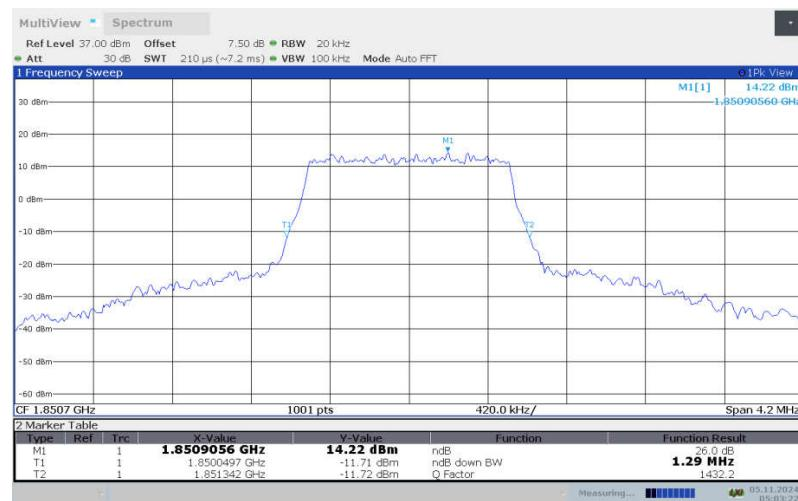
**LTE band 25 , 1.4MHz Bandwidth, LOW, 64QAM (-26dBc BW)**
