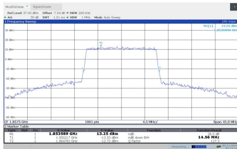
**LTE band 25 , 15MHz Bandwidth, LOW, 64QAM (-26dBc BW)**
