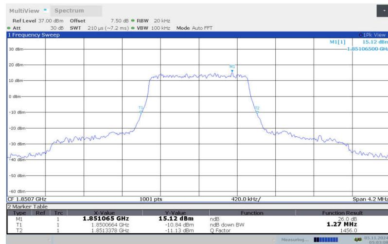
**LTE band 25 , 1.4MHz Bandwidth, LOW, 16QAM (-26dBc BW)**
