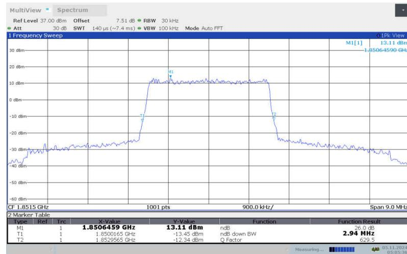
**LTE band 25 , 3MHz Bandwidth, LOW, 16QAM (-26dBc BW)**
