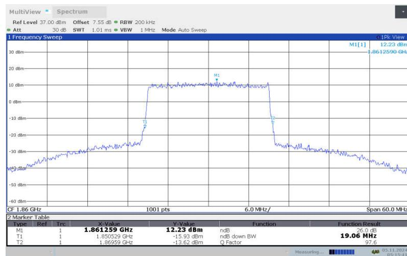
**LTE band 25 , 20MHz Bandwidth, LOW, 64QAM (-26dBc BW)**
