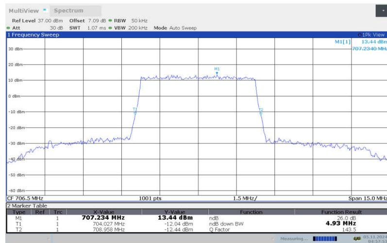
**LTE band 17 , 5MHz Bandwidth, LOW, 16QAM (-26dBc BW)**
