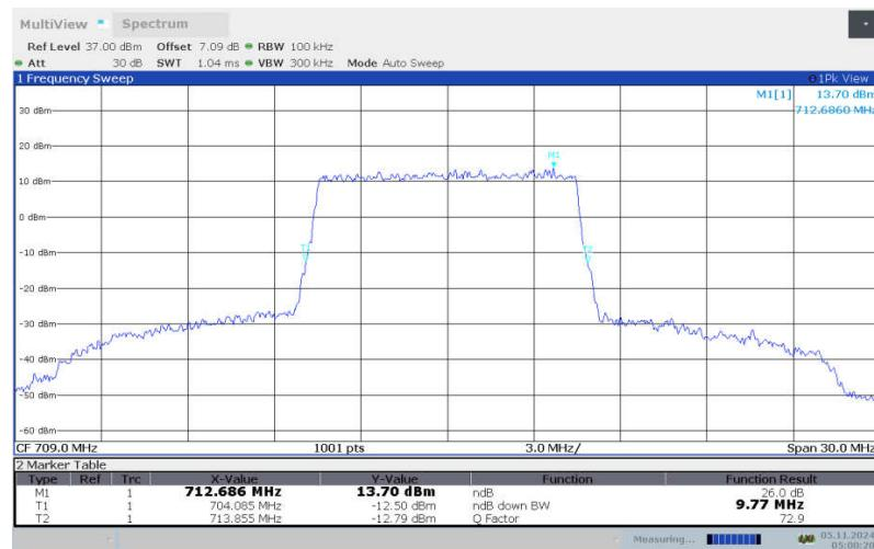
**LTE band 17 , 10MHz Bandwidth, LOW, 16QAM (-26dBc BW)**
