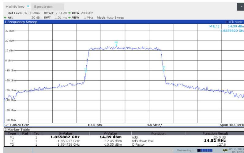
**LTE band 25 , 15MHz Bandwidth, LOW, 16QAM (-26dBc BW)**
