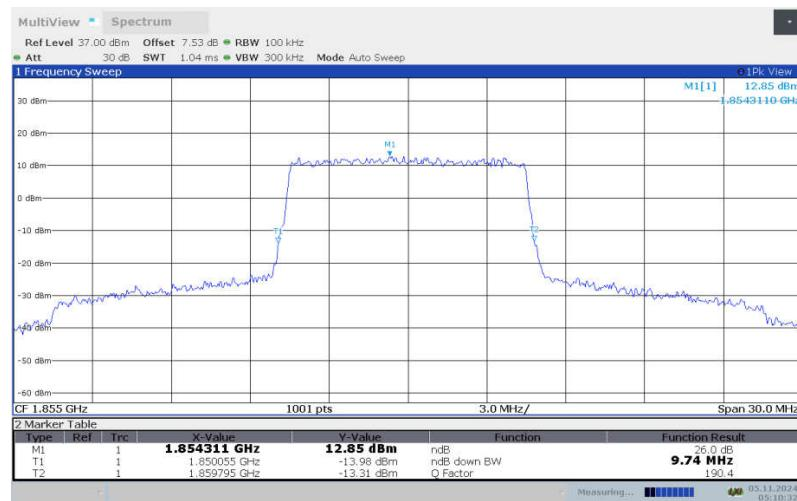
**LTE band 25 , 10MHz Bandwidth, LOW, 16QAM (-26dBc BW)**
