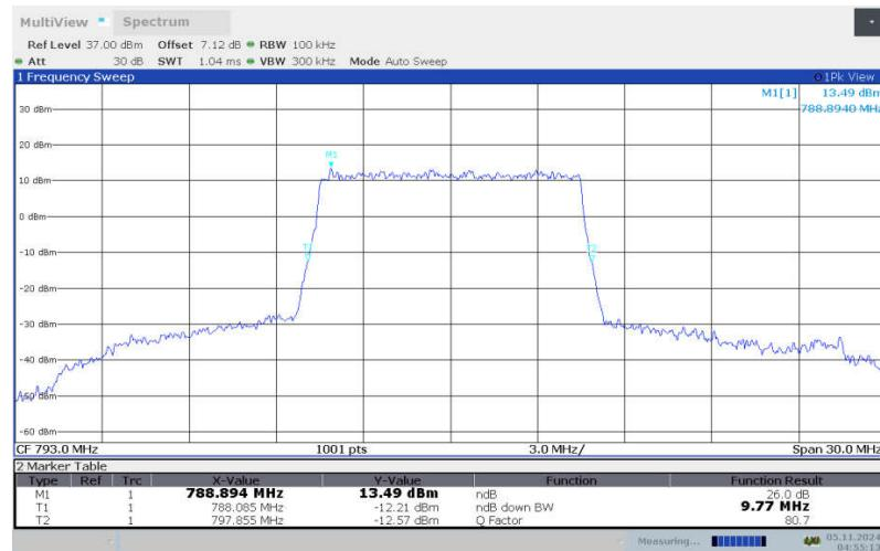
**LTE band 14 , 10MHz Bandwidth, LOW, 16QAM (-26dBc BW)**
