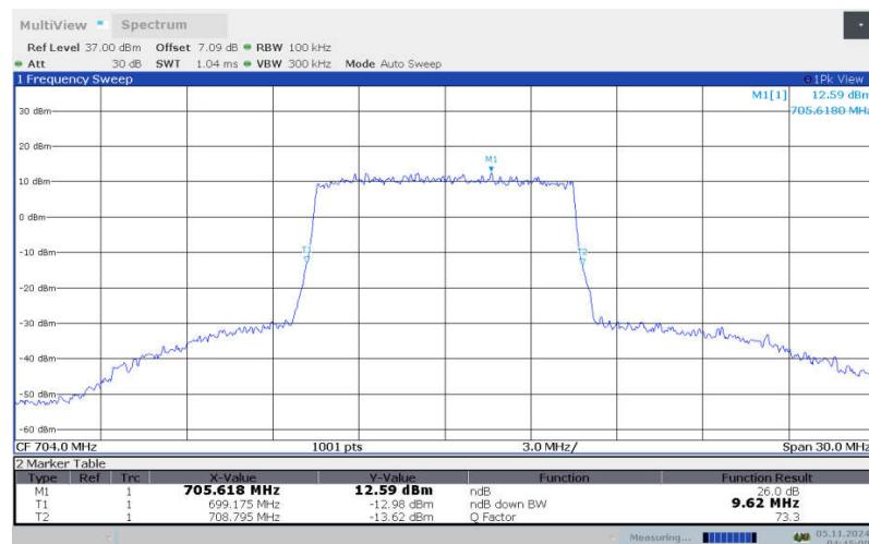
**LTE band 12 , 10MHz Bandwidth, LOW, 64QAM (-26dBc BW)**
