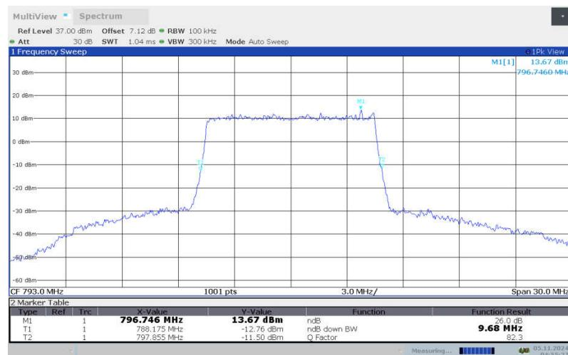
**LTE band 14 , 10MHz Bandwidth, LOW, 64QAM (-26dBc BW)**
