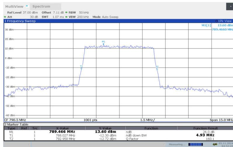
**LTE band 14 , 5MHz Bandwidth, LOW, 16QAM (-26dBc BW)**
