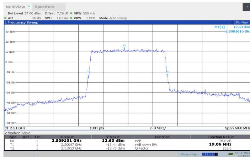
**LTE band 7 , 20MHz Bandwidth, LOW, 16QAM (-26dBc BW)**
