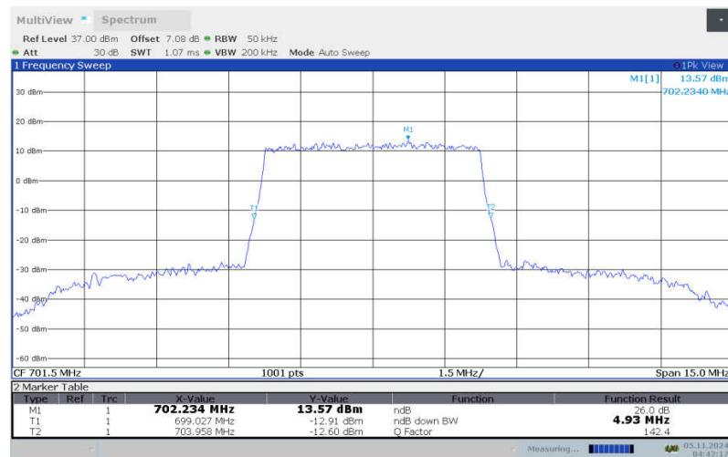
**LTE band 12 , 5MHz Bandwidth, LOW, 16QAM (-26dBc BW)**
