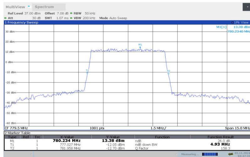
**LTE band 13 , 5MHz Bandwidth, LOW, 16QAM (-26dBc BW)**
