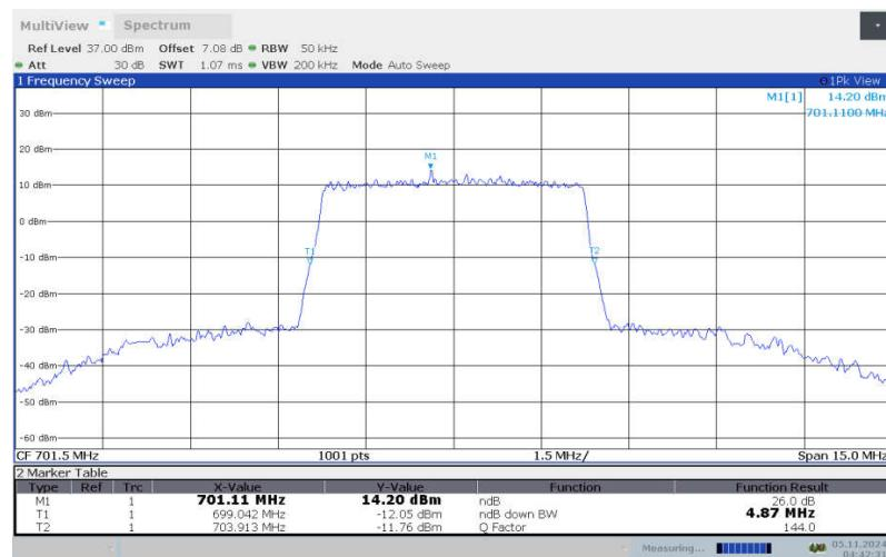
**LTE band 12 , 5MHz Bandwidth, LOW, 64QAM (-26dBc BW)**
