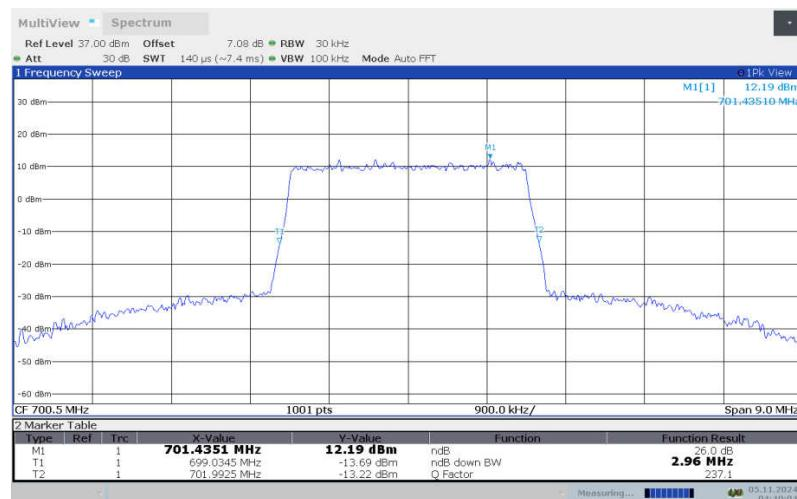
**LTE band 12 , 3MHz Bandwidth, LOW, 64QAM (-26dBc BW)**
