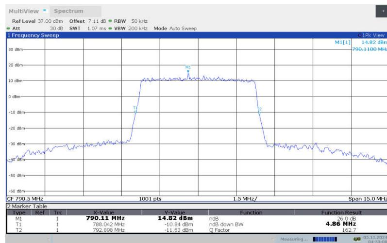
**LTE band 14 , 5MHz Bandwidth, LOW, 64QAM (-26dBc BW)**
