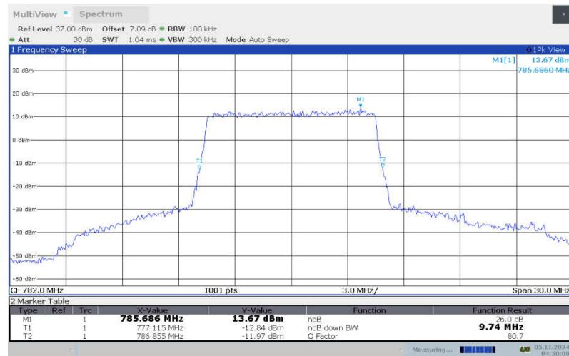
**LTE band 13 , 10MHz Bandwidth, LOW, 16QAM (-26dBc BW)**
