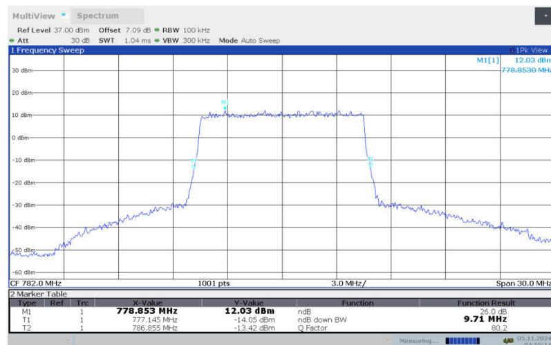
**LTE band 13 , 10MHz Bandwidth, LOW, 64QAM (-26dBc BW)**
