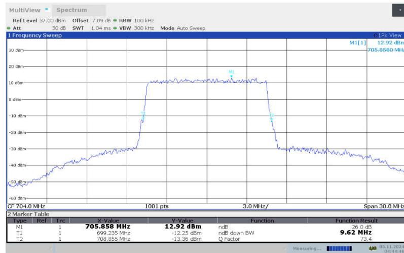
**LTE band 12 , 10MHz Bandwidth, LOW, 16QAM (-26dBc BW)**
