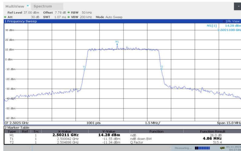
**LTE band 7 , 5MHz Bandwidth, LOW, 64QAM (-26dBc BW)**
