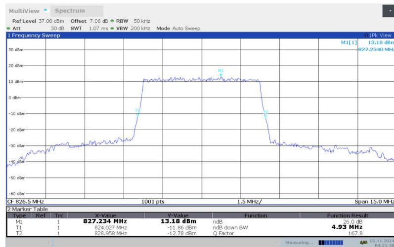
**LTE band 5 , 5MHz Bandwidth, LOW, 16QAM (-26dBc BW)**
