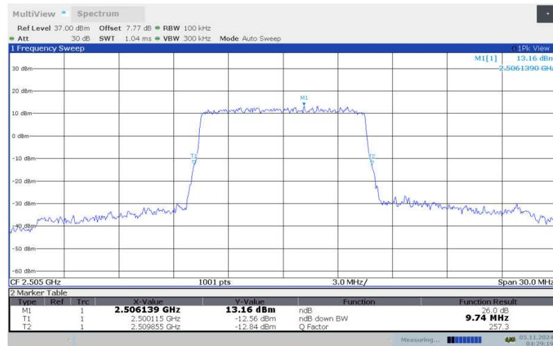
**LTE band 7 , 10MHz Bandwidth, LOW, 16QAM (-26dBc BW)**
