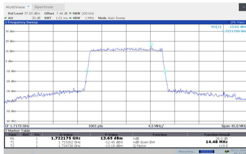
**LTE band 4 , 15MHz Bandwidth, LOW, 64QAM (-26dBc BW)**
