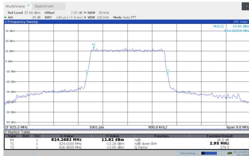
**LTE band 5 , 3MHz Bandwidth, LOW, 16QAM (-26dBc BW)**
