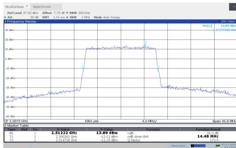
**LTE band 7 , 15MHz Bandwidth, LOW, 64QAM (-26dBc BW)**
