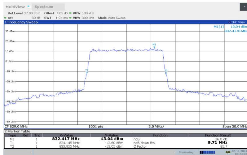
**LTE band 5 , 10MHz Bandwidth, LOW, 16QAM (-26dBc BW)**
