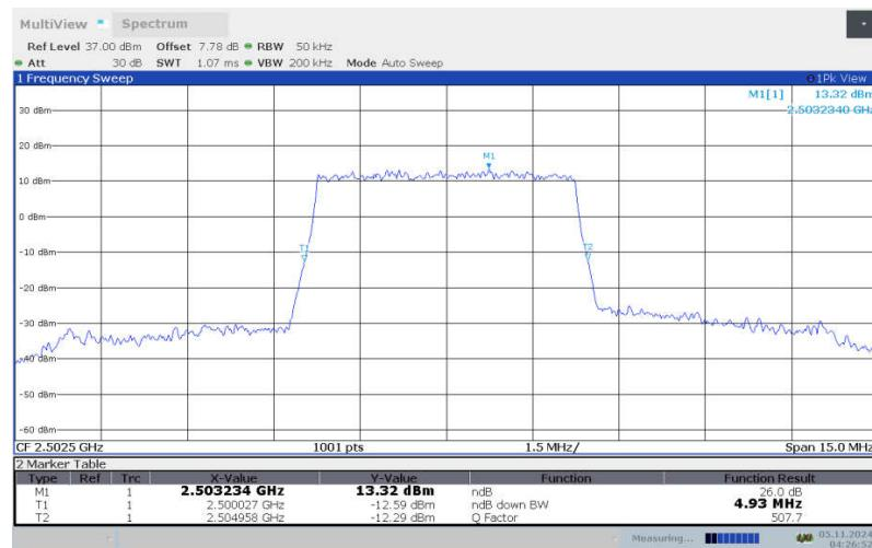
**LTE band 7 , 5MHz Bandwidth, LOW, 16QAM (-26dBc BW)**
