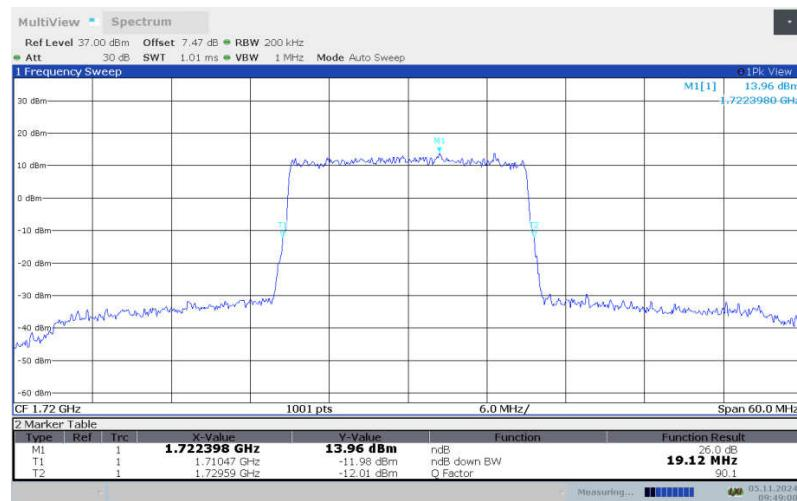
**LTE band 4 , 20MHz Bandwidth, LOW, 16QAM (-26dBc BW)**
