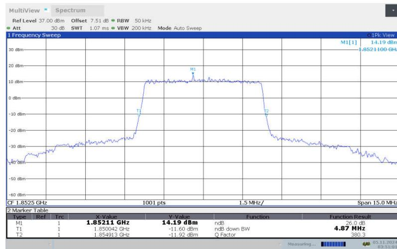
**LTE band 2 , 5MHz Bandwidth, LOW, 64QAM (-26dBc BW)**
