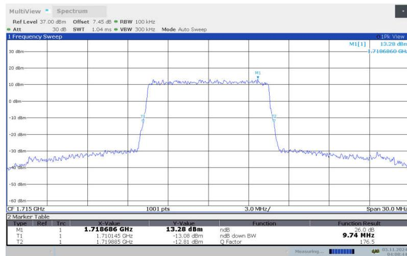
**LTE band 4 , 10MHz Bandwidth, LOW, 16QAM (-26dBc BW)**
