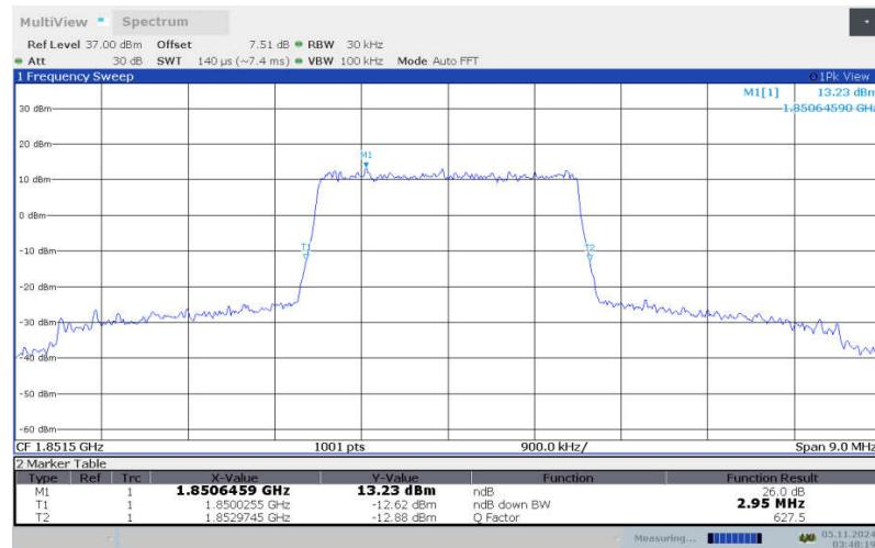
**LTE band 2 , 3MHz Bandwidth, LOW, 16QAM (-26dBc BW)**
