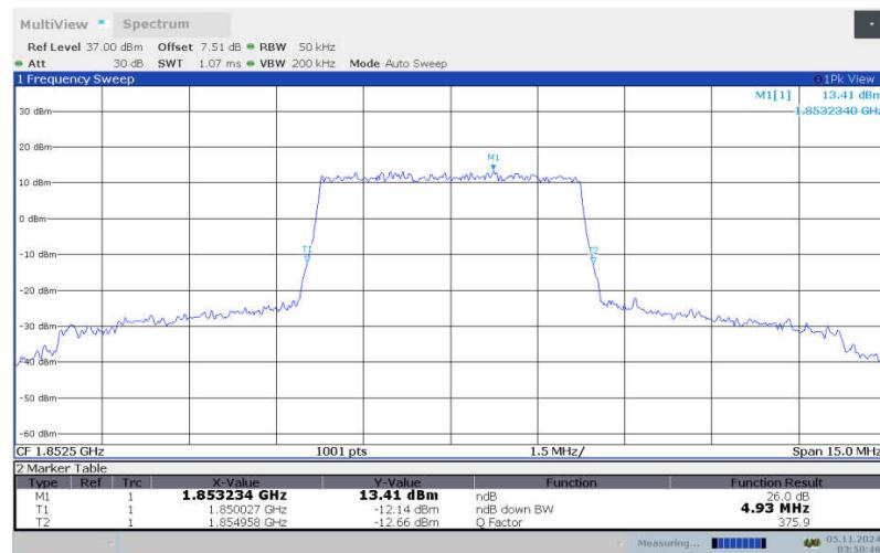
**LTE band 2 , 5MHz Bandwidth, LOW, 16QAM (-26dBc BW)**
