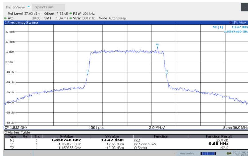
**LTE band 2 , 10MHz Bandwidth, LOW, 64QAM (-26dBc BW)**
