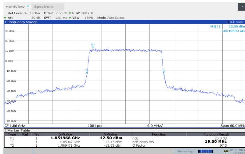
**LTE band 2 , 20MHz Bandwidth, LOW, 16QAM (-26dBc BW)**
