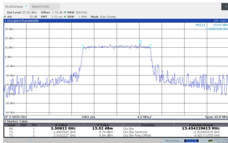
**LTE band 41 , 15MHz Bandwidth, LOW, 64QAM (99% BW)**
