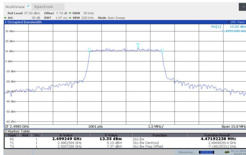
**LTE band 41 , 5MHz Bandwidth, LOW, 16QAM (99% BW)**
