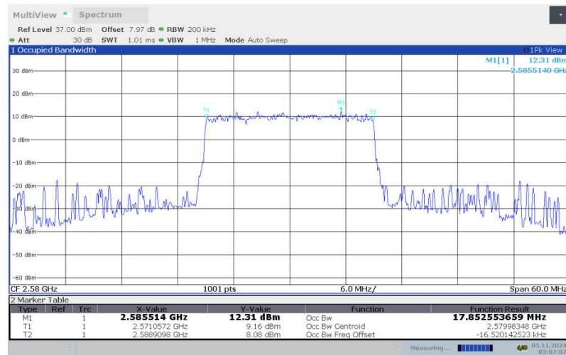
**LTE band 38 , 20MHz Bandwidth, LOW, 64QAM (99% BW)**
