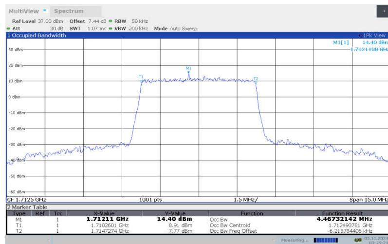
**LTE band 66 , 5MHz Bandwidth, LOW, 64QAM (99% BW)**
