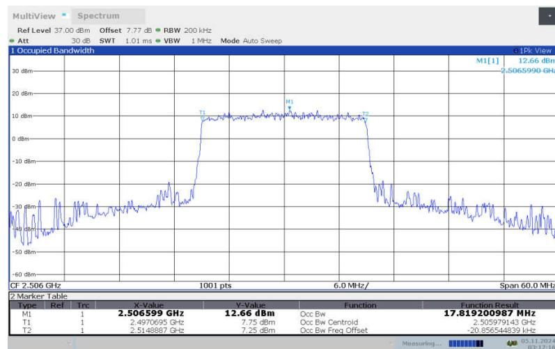
**LTE band 41 , 20MHz Bandwidth, LOW, 64QAM (99% BW)**
