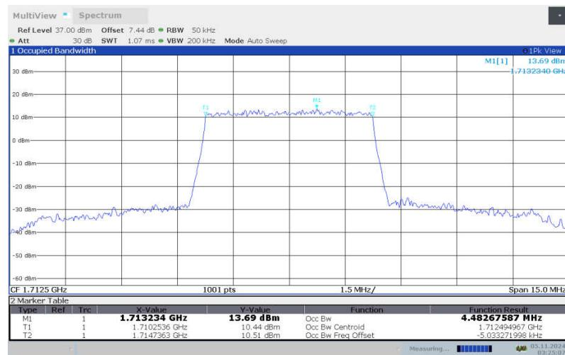
**LTE band 66 , 5MHz Bandwidth, LOW, 16QAM (99% BW)**
