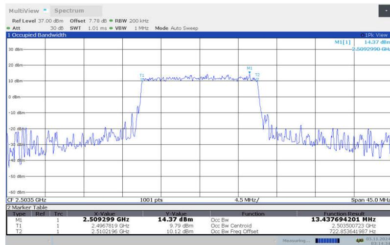
**LTE band 41 , 15MHz Bandwidth, LOW, 16QAM (99% BW)**
