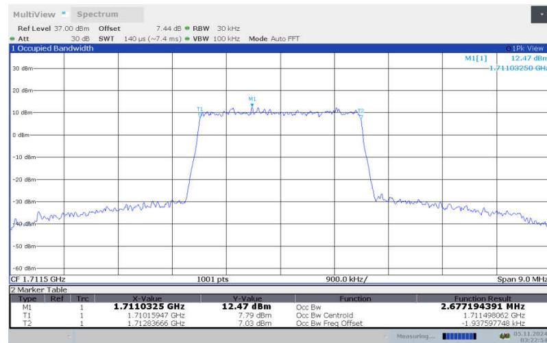
**LTE band 66 , 3MHz Bandwidth, LOW, 64QAM (99% BW)**
