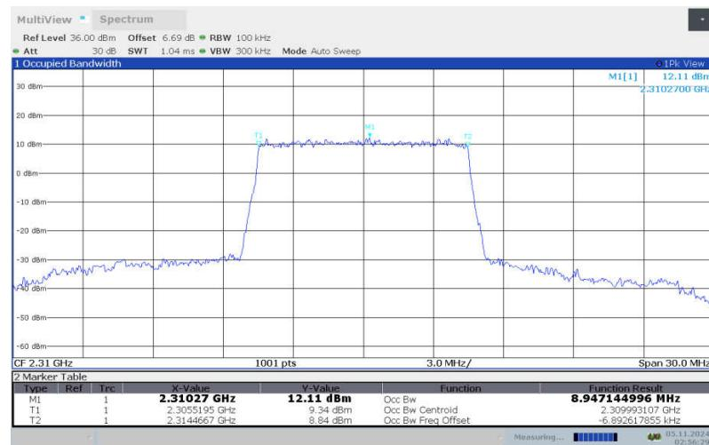
**LTE band 30 , 10MHz Bandwidth, LOW, 16QAM (99% BW)**
