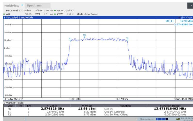
**LTE band 38 , 15MHz Bandwidth, LOW, 64QAM (99% BW)**
