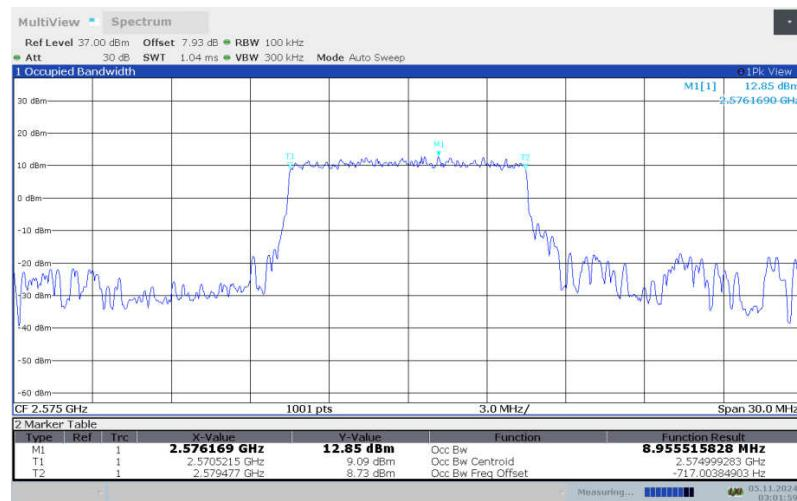
**LTE band 38 , 10MHz Bandwidth, LOW, 16QAM (99% BW)**
