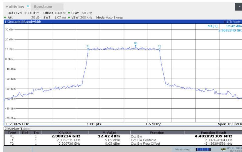
**LTE band 30 , 5MHz Bandwidth, LOW, 16QAM (99% BW)**
