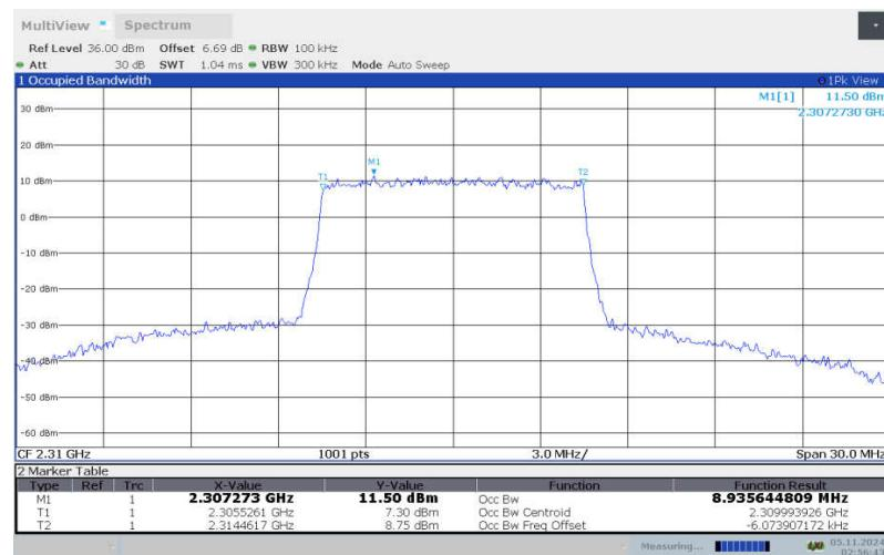
**LTE band 30 , 10MHz Bandwidth, LOW, 64QAM (99% BW)**
