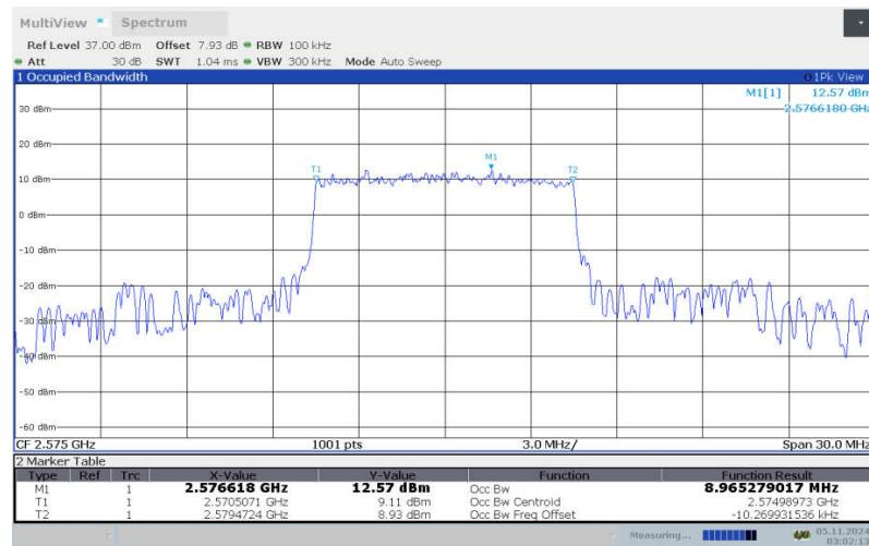
**LTE band 38 , 10MHz Bandwidth, LOW, 64QAM (99% BW)**
