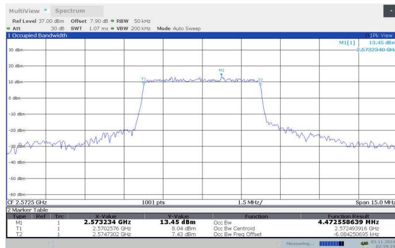
**LTE band 38 , 5MHz Bandwidth, LOW, 16QAM (99% BW)**
