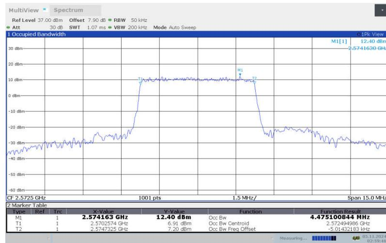
**LTE band 38 , 5MHz Bandwidth, LOW, 64QAM (99% BW)**
