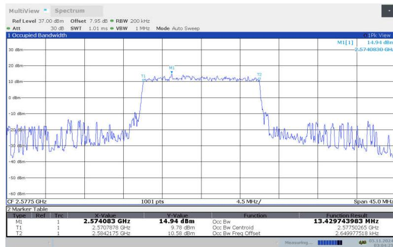
**LTE band 38 , 15MHz Bandwidth, LOW, 16QAM (99% BW)**
