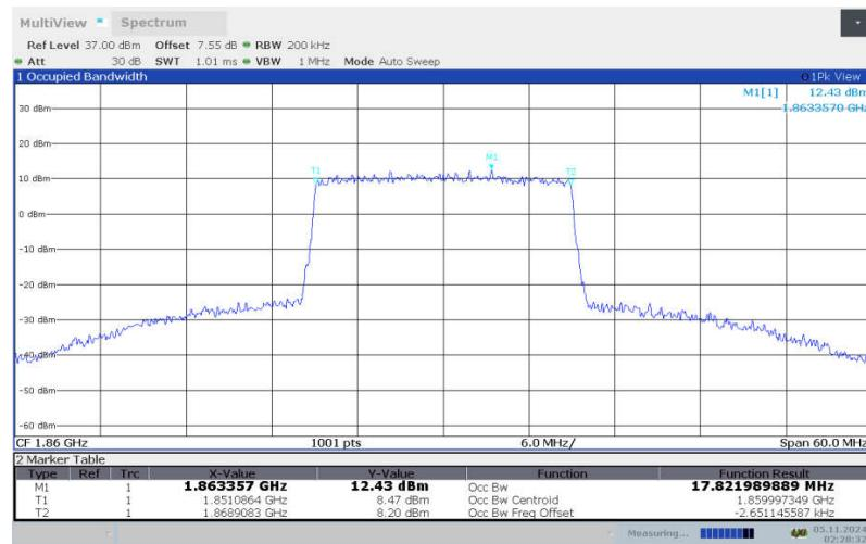
**LTE band 25 , 20MHz Bandwidth, LOW, 64QAM (99% BW)**
