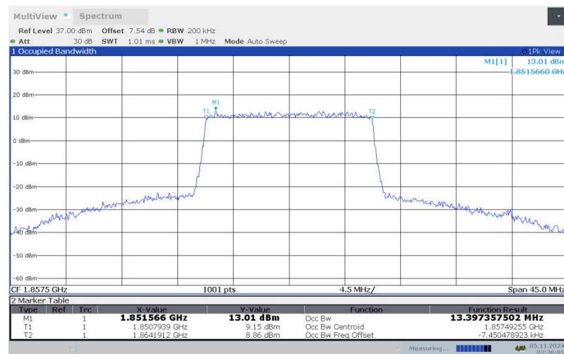
**LTE band 25 , 15MHz Bandwidth, LOW, 64QAM (99% BW)**
