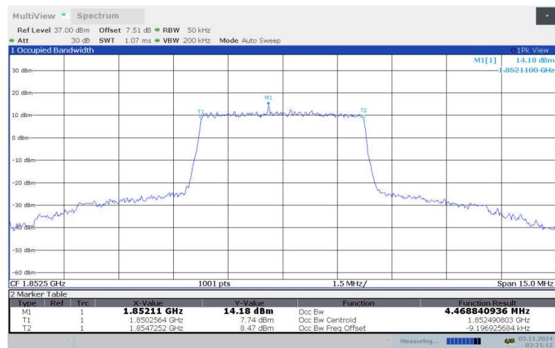
**LTE band 25 , 5MHz Bandwidth, LOW, 64QAM (99% BW)**
