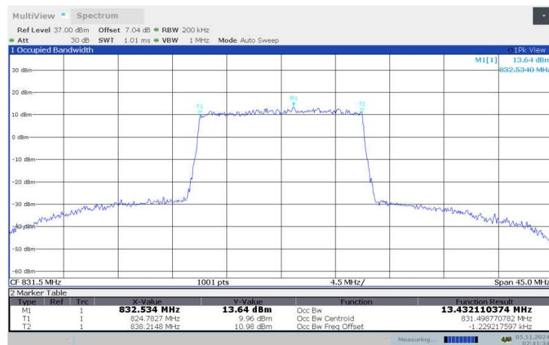
**LTE band 26 , 15MHz Bandwidth, LOW, 64QAM (99% BW)**
