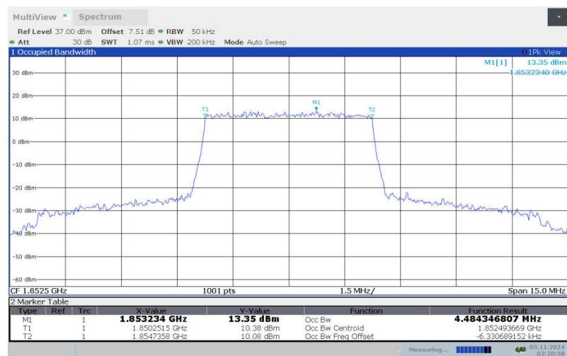
**LTE band 25 , 5MHz Bandwidth, LOW, 16QAM (99% BW)**
