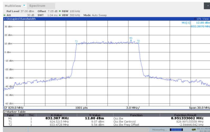
**LTE band 26 , 10MHz Bandwidth, LOW, 16QAM (99% BW)**
