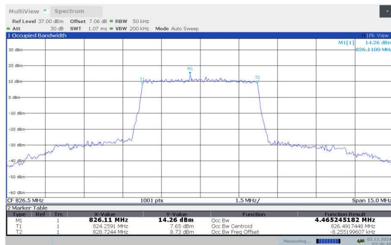
**LTE band 26 , 5MHz Bandwidth, LOW, 64QAM (99% BW)**
