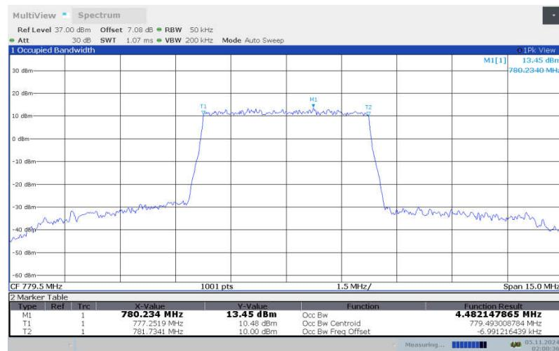
**LTE band 13 , 5MHz Bandwidth, LOW, 16QAM (99% BW)**
