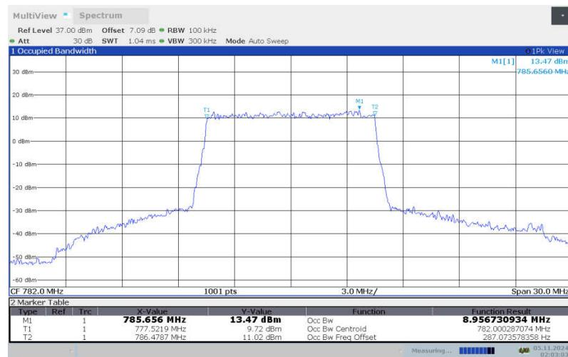
**LTE band 13 , 10MHz Bandwidth, LOW, 16QAM (99% BW)**
