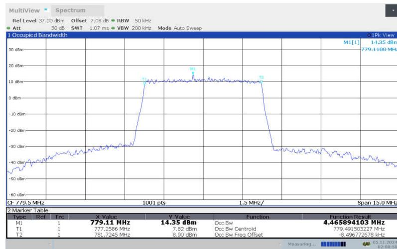
**LTE band 13 , 5MHz Bandwidth, LOW, 64QAM (99% BW)**
