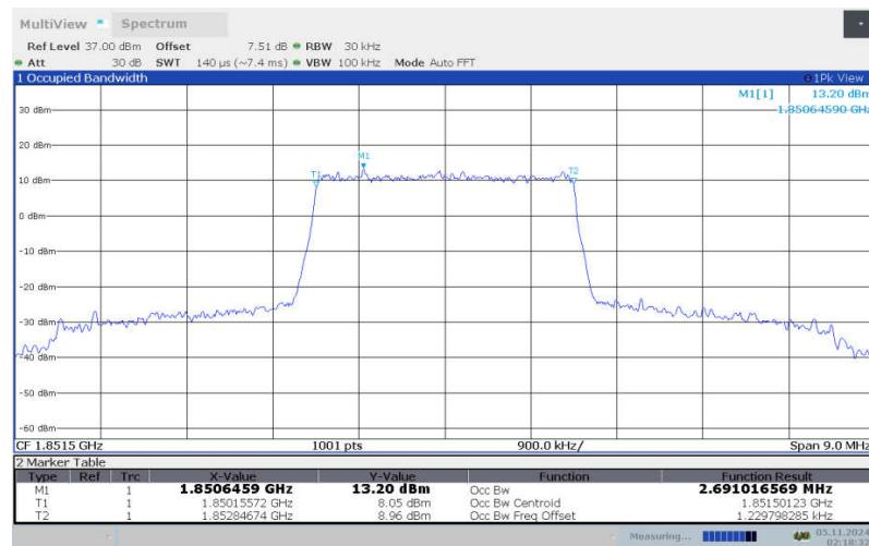
**LTE band 25 , 3MHz Bandwidth, LOW, 16QAM (99% BW)**
