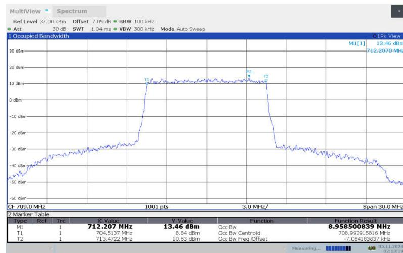
**LTE band 17 , 10MHz Bandwidth, LOW, 16QAM (99% BW)**
