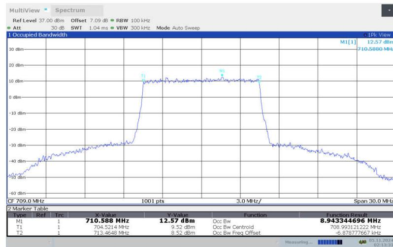
**LTE band 17 , 10MHz Bandwidth, LOW, 64QAM (99% BW)**
