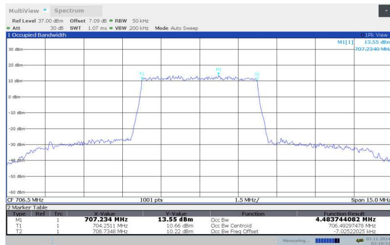
**LTE band 17 , 5MHz Bandwidth, LOW, 16QAM (99% BW)**
