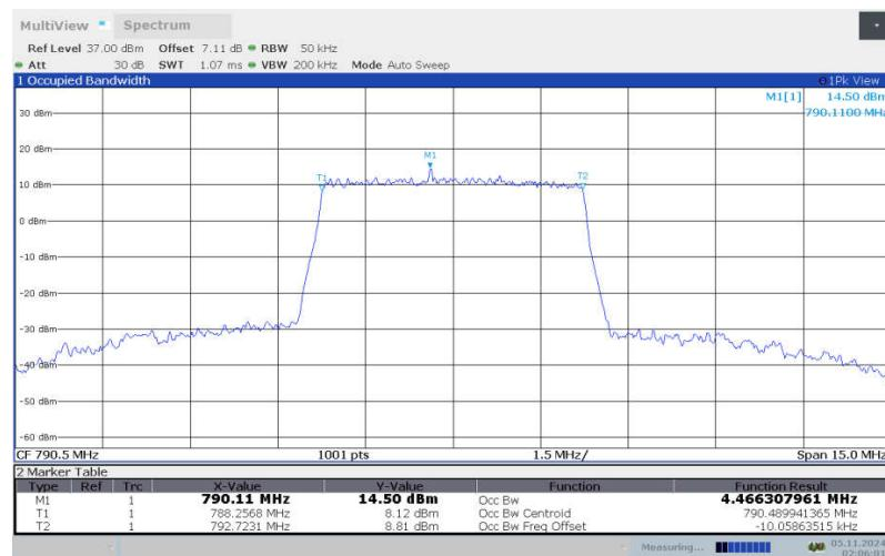
**LTE band 14 , 5MHz Bandwidth, LOW, 64QAM (99% BW)**
