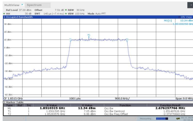
**LTE band 25 , 3MHz Bandwidth, LOW, 64QAM (99% BW)**
