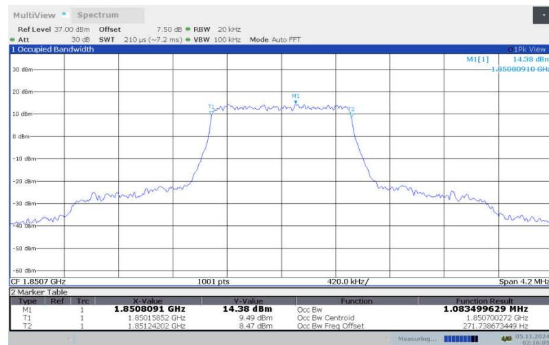
**LTE band 25 , 1.4MHz Bandwidth, LOW, 16QAM (99% BW)**
