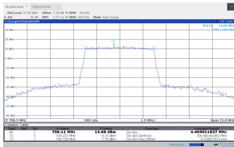
**LTE band 17 , 5MHz Bandwidth, LOW, 64QAM (99% BW)**
