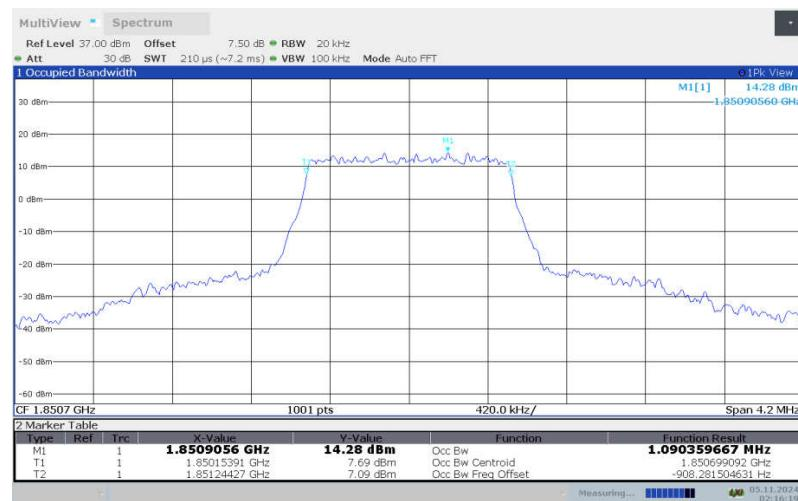
**LTE band 25 , 1.4MHz Bandwidth, LOW, 64QAM (99% BW)**
