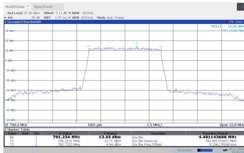
**LTE band 14 , 5MHz Bandwidth, LOW, 16QAM (99% BW)**
