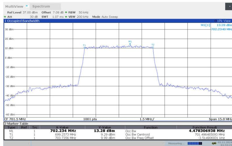
**LTE band 12 , 5MHz Bandwidth, LOW, 16QAM (99% BW)**
