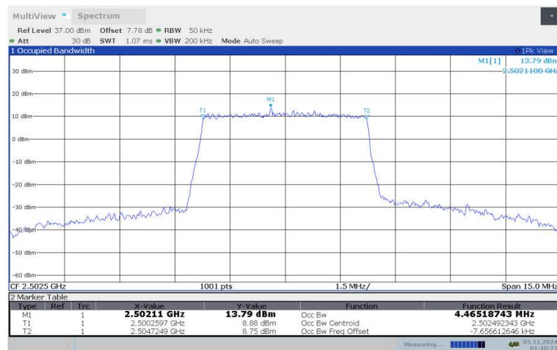
**LTE band 7 , 5MHz Bandwidth, LOW, 64QAM (99% BW)**
