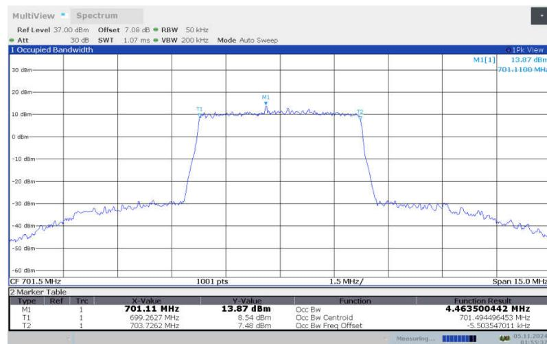
**LTE band 12 , 5MHz Bandwidth, LOW, 64QAM (99% BW)**
