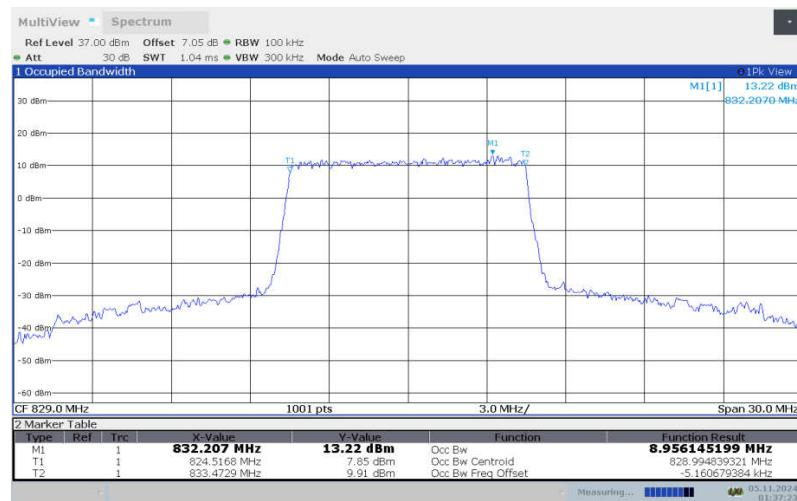
**LTE band 5 , 10MHz Bandwidth, LOW, 16QAM (99% BW)**
