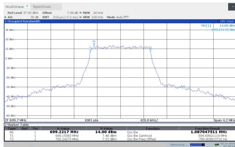
**LTE band 12 , 1.4MHz Bandwidth, LOW, 64QAM (99% BW)**
