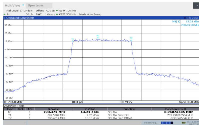
**LTE band 12 , 10MHz Bandwidth, LOW, 16QAM (99% BW)**
