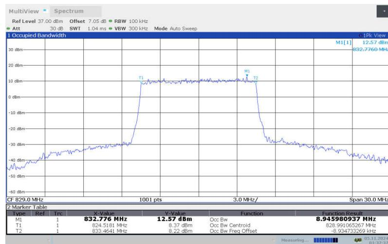
**LTE band 5 , 10MHz Bandwidth, LOW, 64QAM (99% BW)**
