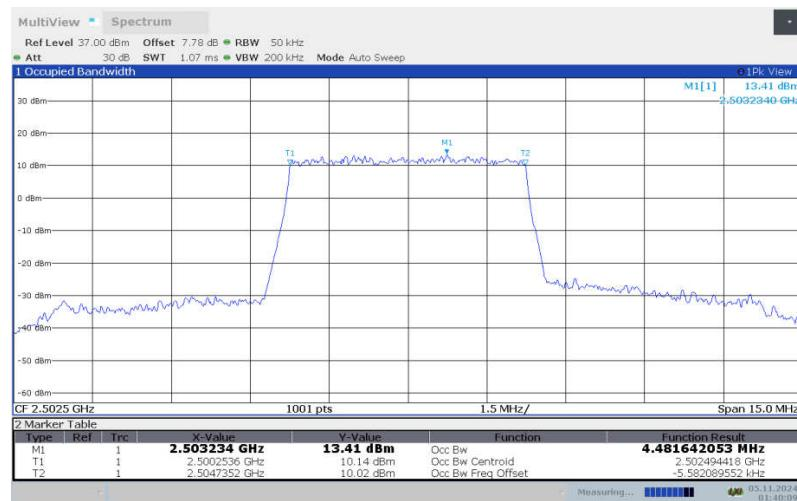
**LTE band 7 , 5MHz Bandwidth, LOW, 16QAM (99% BW)**
