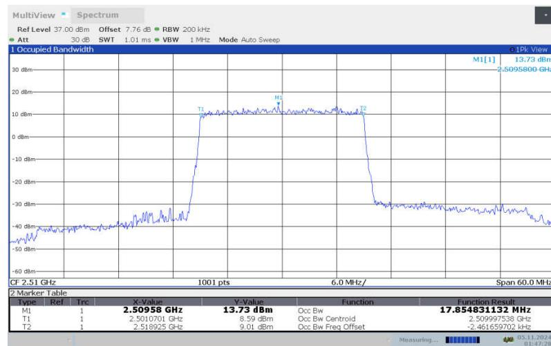
**LTE band 7 , 20MHz Bandwidth, LOW, 16QAM (99% BW)**
