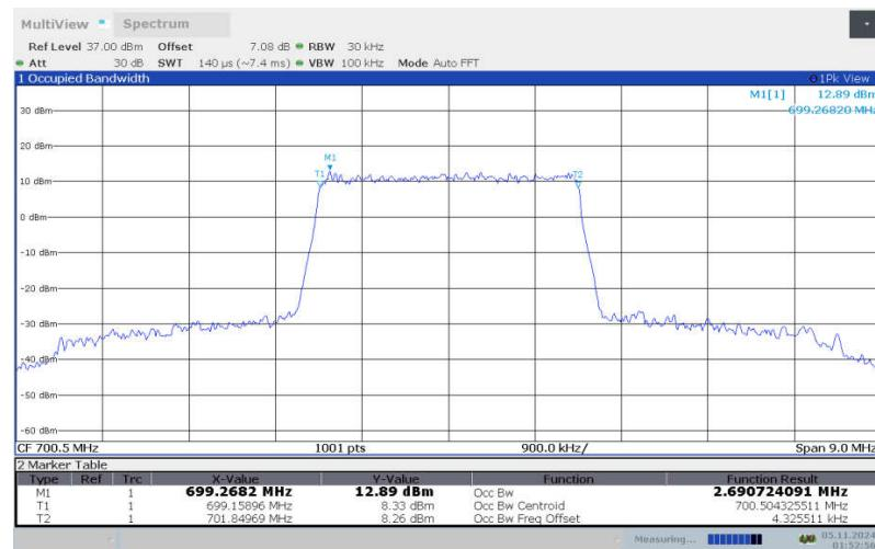
**LTE band 12 , 3MHz Bandwidth, LOW, 16QAM (99% BW)**
