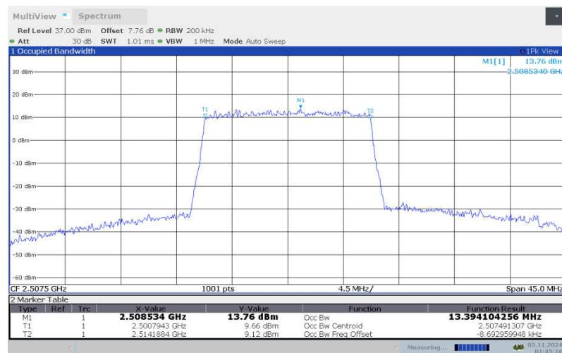
**LTE band 7 , 15MHz Bandwidth, LOW, 64QAM (99% BW)**
