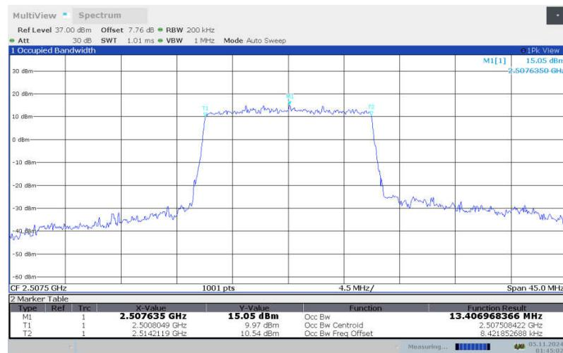
**LTE band 7 , 15MHz Bandwidth, LOW, 16QAM (99% BW)**
