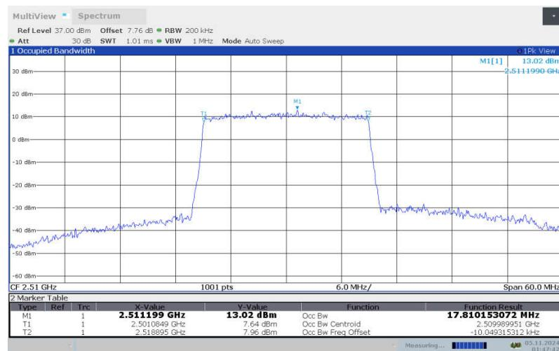
**LTE band 7 , 20MHz Bandwidth, LOW, 64QAM (99% BW)**
