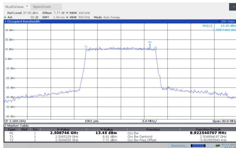
**LTE band 7 , 10MHz Bandwidth, LOW, 64QAM (99% BW)**
