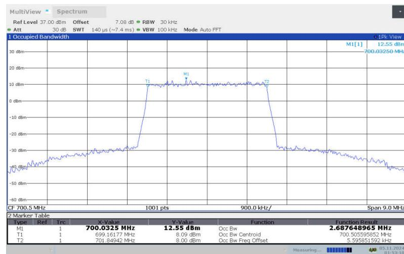
**LTE band 12 , 3MHz Bandwidth, LOW, 64QAM (99% BW)**
