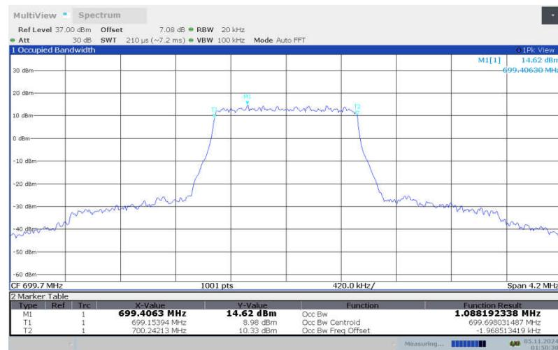
**LTE band 12 , 1.4MHz Bandwidth, LOW, 16QAM (99% BW)**
