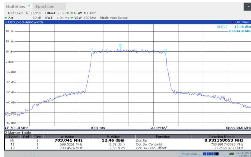
**LTE band 12 , 10MHz Bandwidth, LOW, 64QAM (99% BW)**
