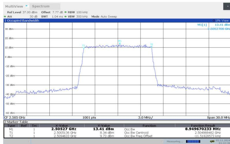
**LTE band 7 , 10MHz Bandwidth, LOW, 16QAM (99% BW)**
