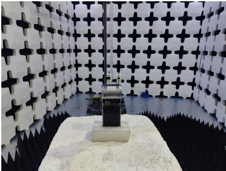
18. Radiated Emissions (Par22/24/27, 26.5GHz-40GHz)
