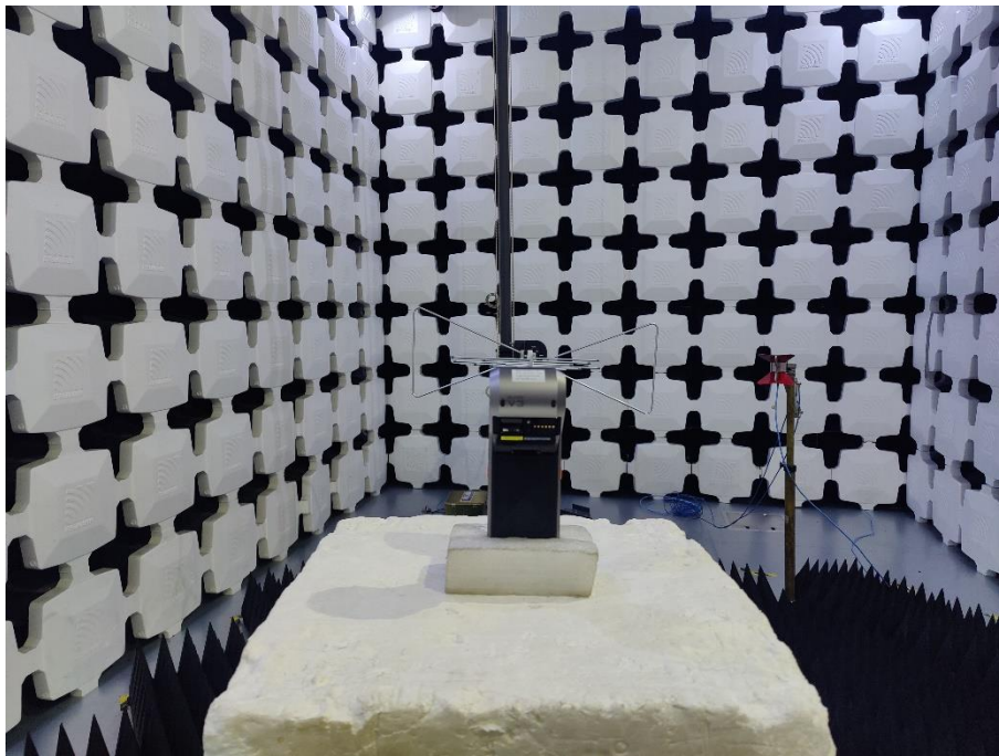
16. Radiated Emissions (Part 22/24/27, 30MHz-18GHz)
