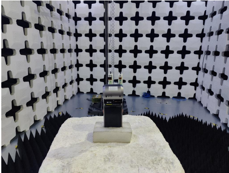
15. Radiated Emissions (Part 15C&Part 15E, 26.5GHz-40GHz)
