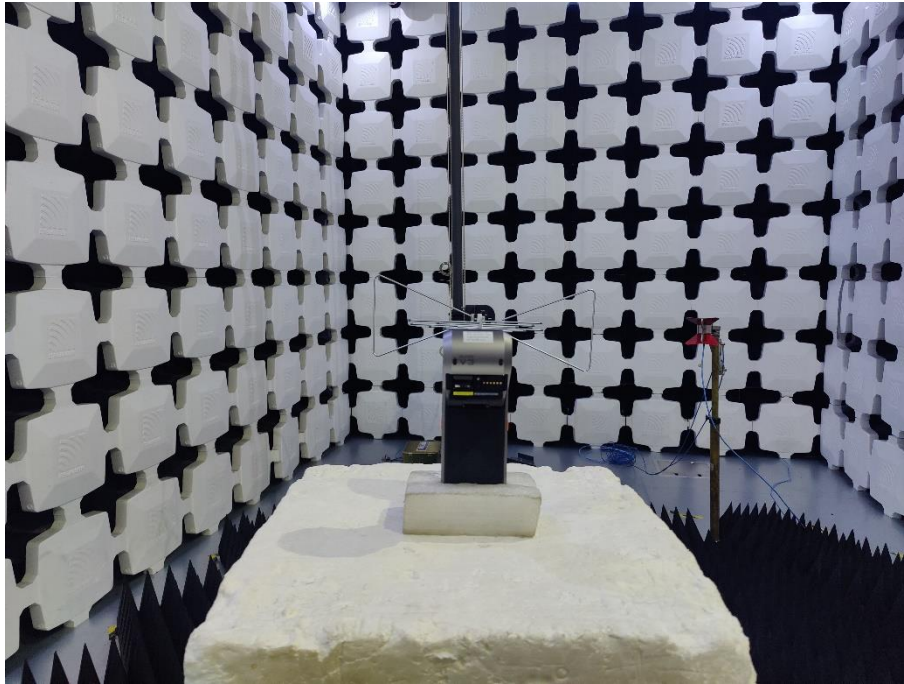
13. Radiated Emissions (Part 15C&Part 15E, 1GHz -18GHz)
