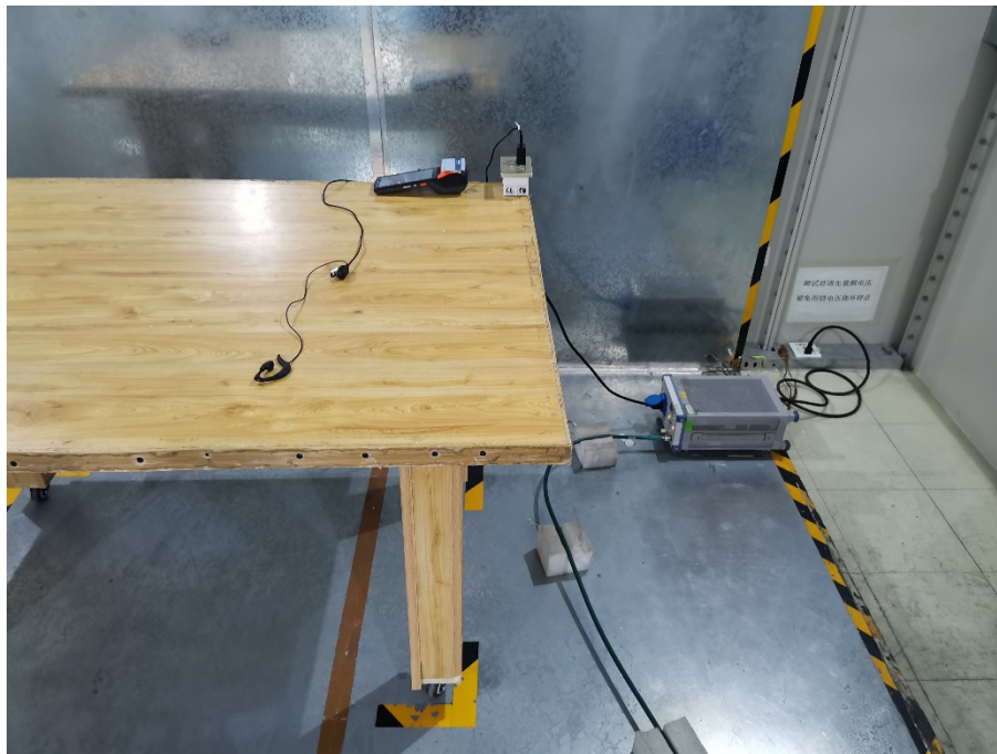
Conducted Emissions Side View
