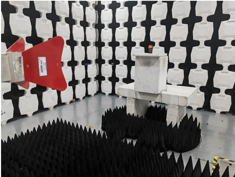
Description: Radiated Emission Test Setup (1GHz -18GHz)
