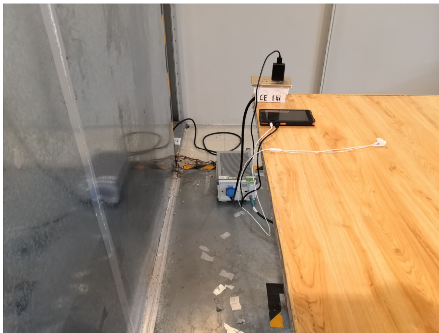
Conducted Emissions (Side View)
