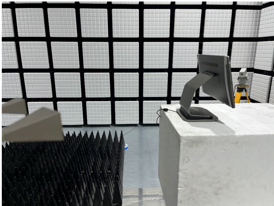
Description: Radiated Emission Test Setup (Above 18GHz)
