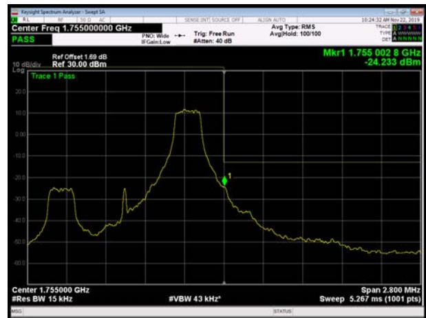
LTE Band 4 QPSK 1.4MHz CH-High, 100%RB
