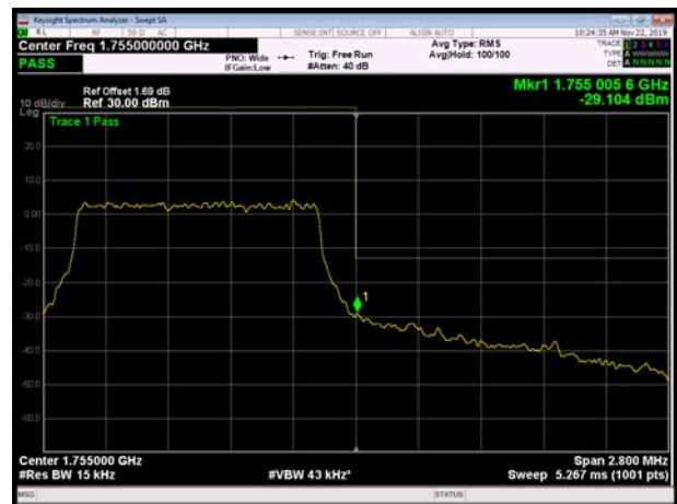
LTE Band 4 QPSK 3MHz CH-High, 1 RB
