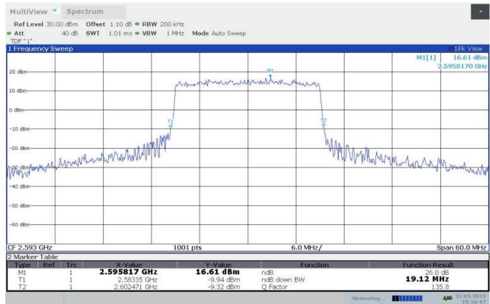
**LTE band 41 , 20MHz Bandwidth,MID,16QAM (-26dBc BW)**
