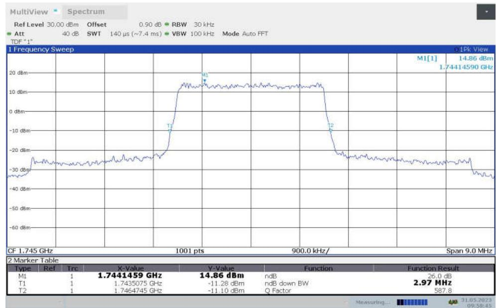
**LTE band 66 , 3MHz Bandwidth,MID,16QAM (-26dBc BW)**
