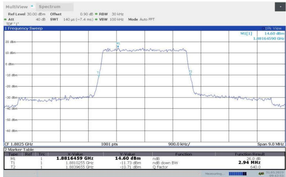
**LTE band 25 , 3MHz Bandwidth,MID,16QAM (-26dBc BW)**
