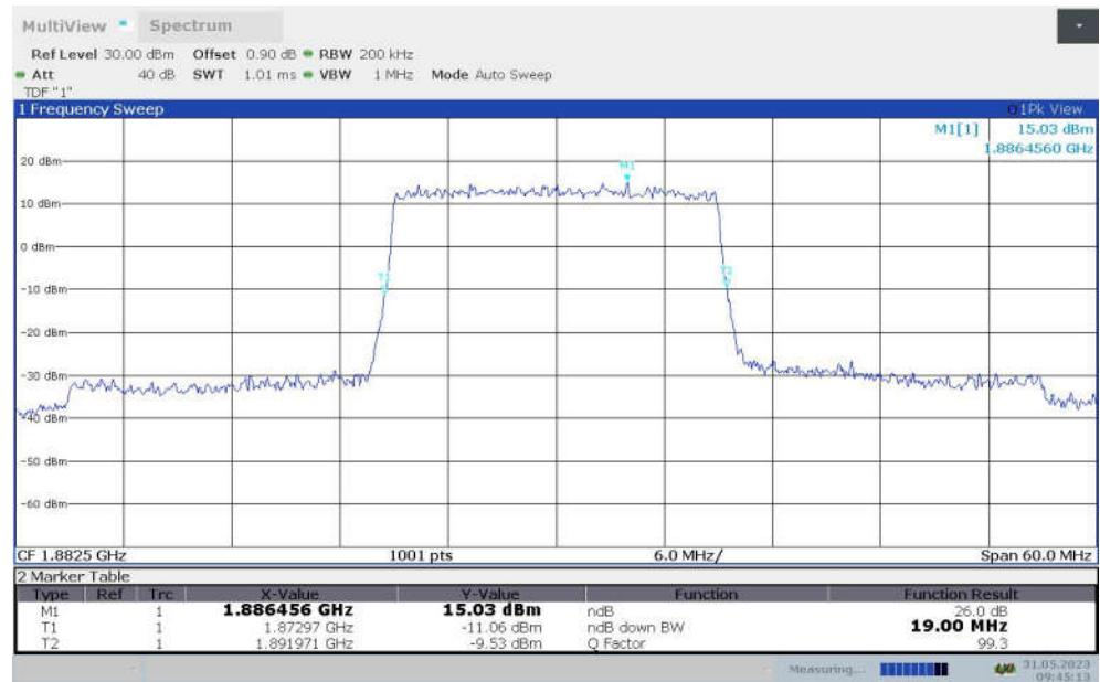
**LTE band 25 , 20MHz Bandwidth,MID,16QAM (-26dBc BW)**
