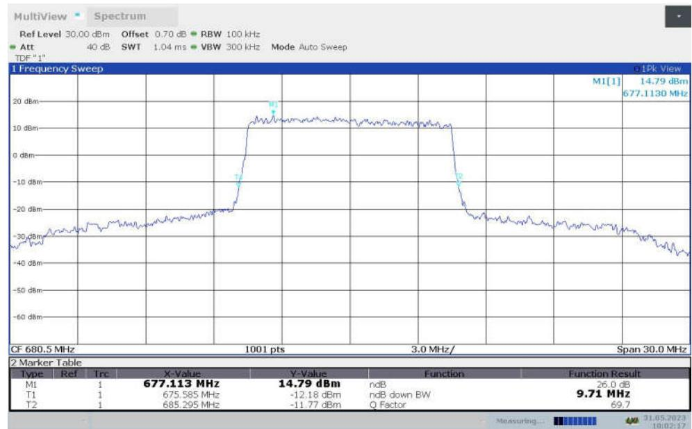
**LTE band 71 , 10MHz Bandwidth,MID,16QAM (-26dBc BW)**
