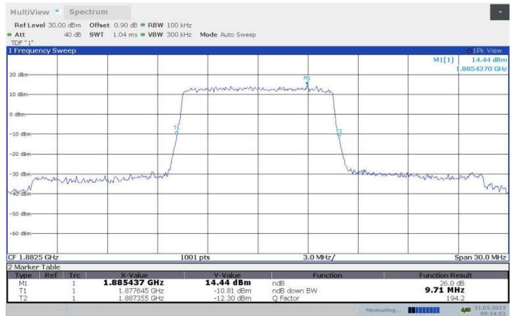
**LTE band 25 , 10MHz Bandwidth,MID,16QAM (-26dBc BW)**
