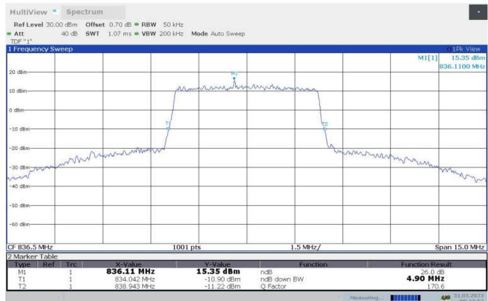
**LTE band 26 (824 MHz-849 MHz),10MHz(-26dBc)**
