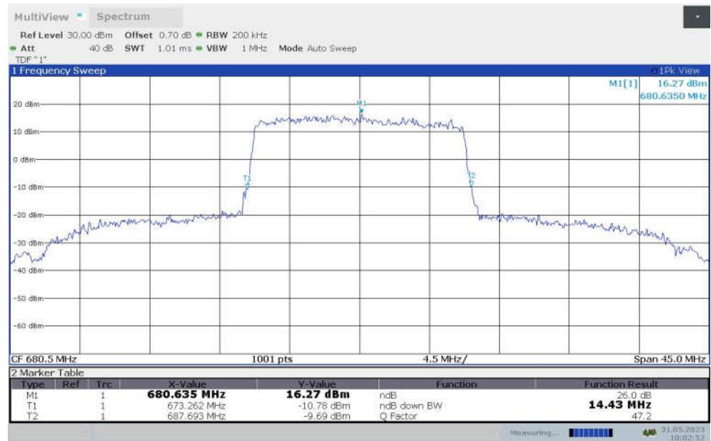
**LTE band 71 , 15MHz Bandwidth,MID,16QAM (-26dBc BW)**
