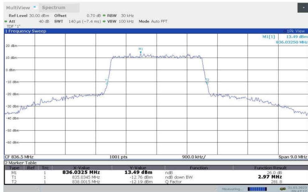
**LTE band 26 (824 MHz-849 MHz),5MHz(-26dBc)**
