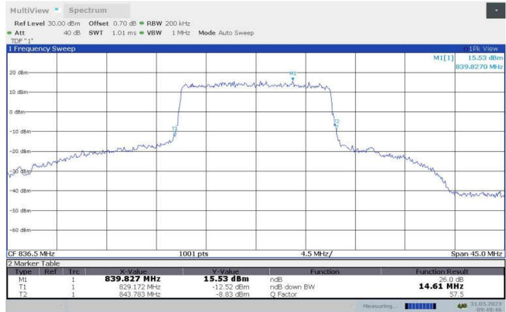
**LTE band 26 , 15MHz Bandwidth,MID,16QAM (-26dBc BW)**
