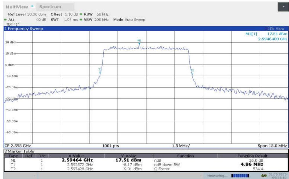
**LTE band 38 , 5MHz Bandwidth,MID,16QAM (-26dBc BW)**
