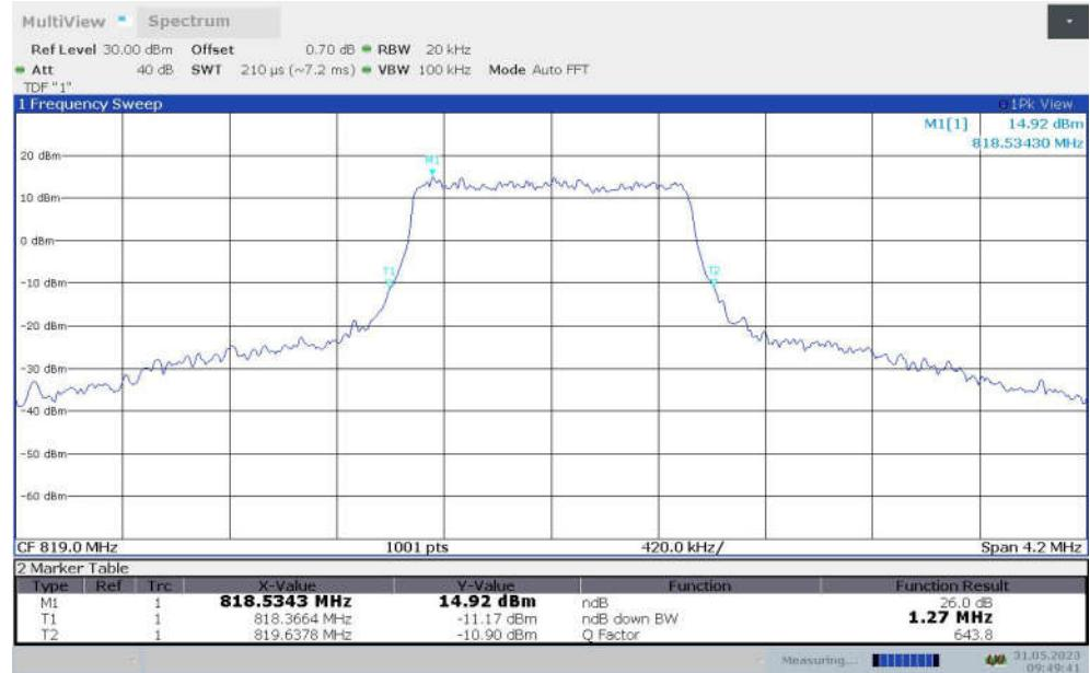
**LTE band 26 (814 MHz-824 MHz),3MHz(-26dBc)**
