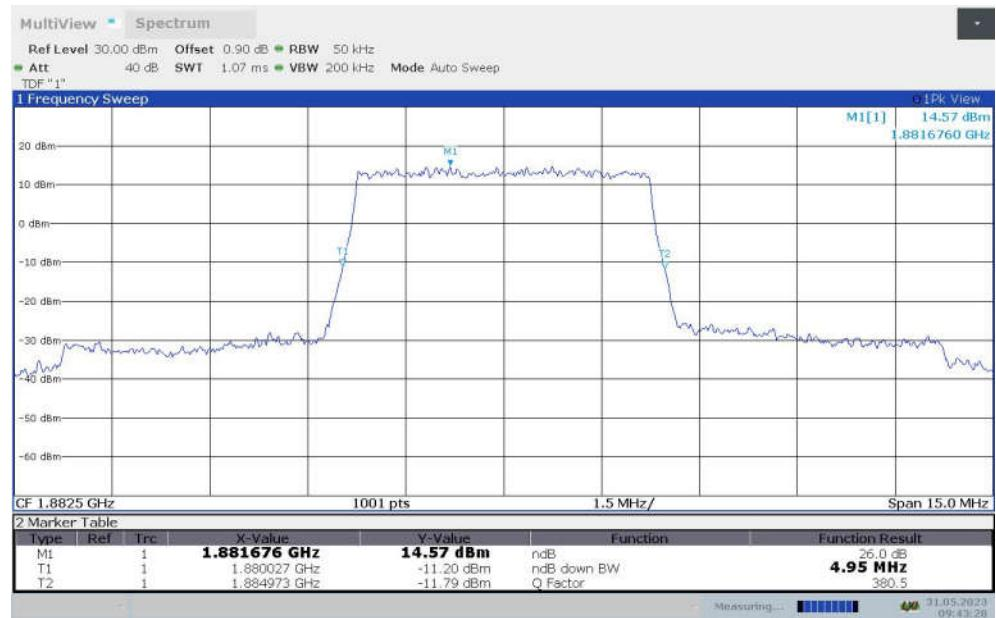
**LTE band 25 , 5MHz Bandwidth,MID,16QAM (-26dBc BW)**
