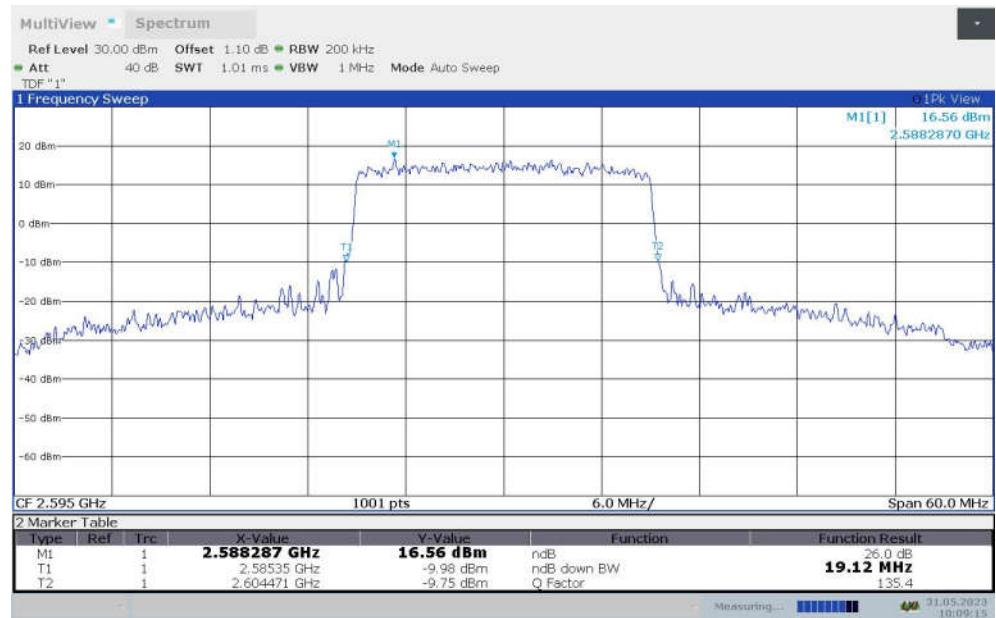
**LTE band 38 , 20MHz Bandwidth,MID,16QAM (-26dBc BW)**
