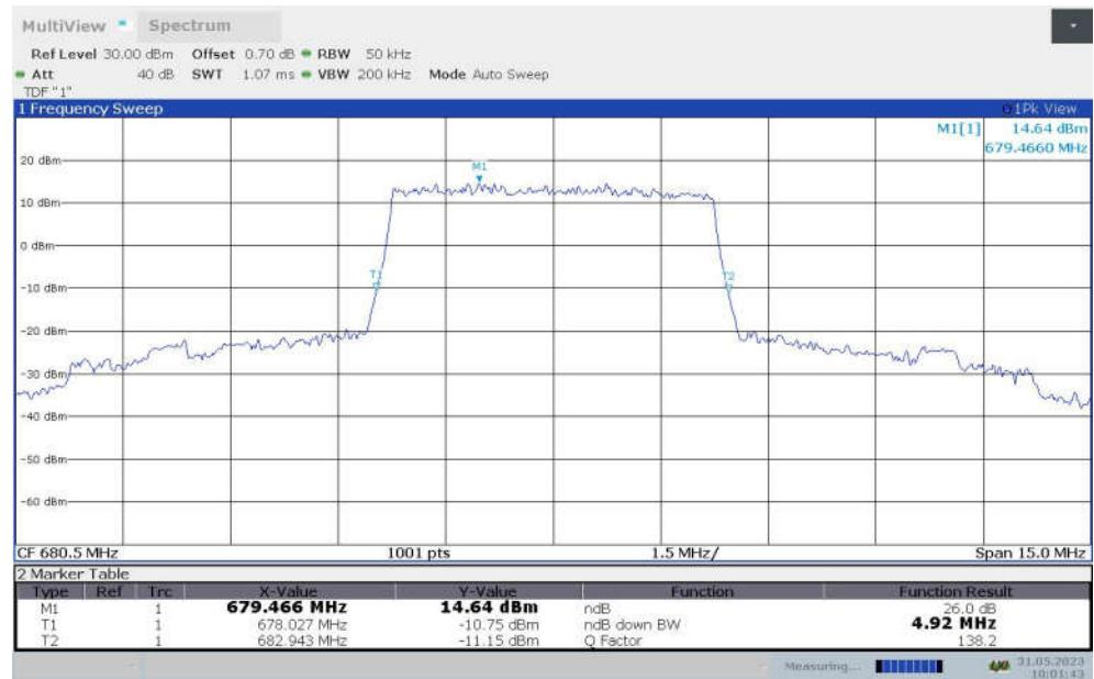
**LTE band 71 , 5MHz Bandwidth,MID,16QAM (-26dBc BW)**
