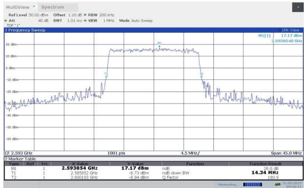
**LTE band 41 , 15MHz Bandwidth,MID,16QAM (-26dBc BW)**
