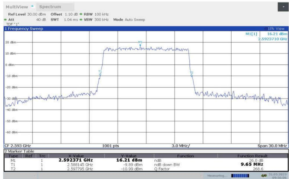
**LTE band 41 , 10MHz Bandwidth,MID,16QAM (-26dBc BW)**
