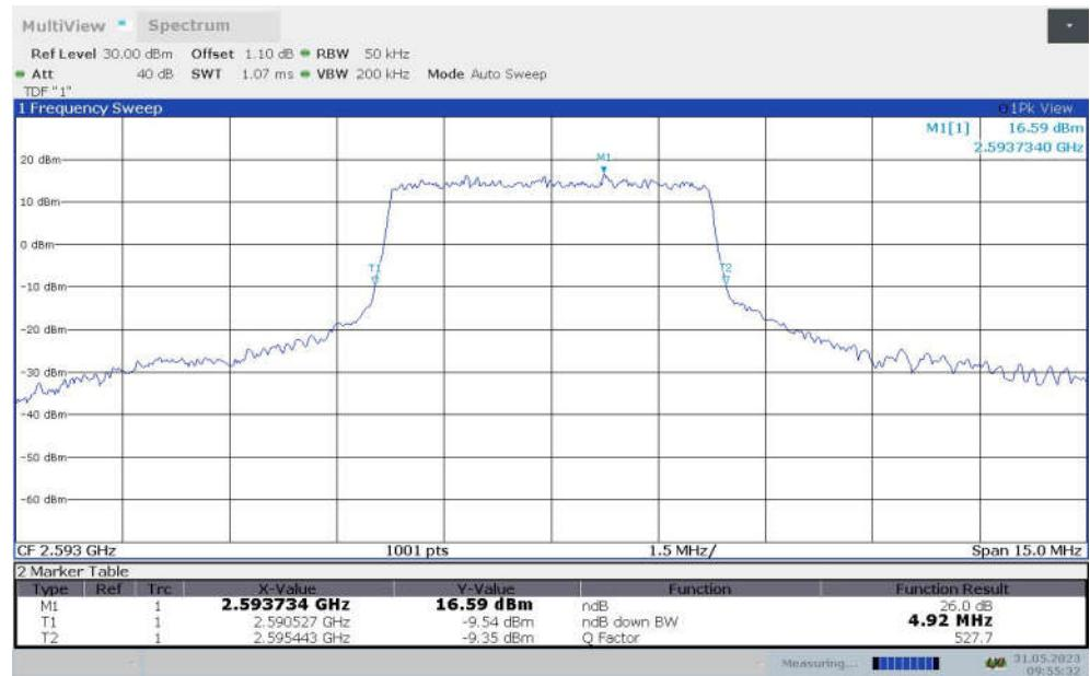
**LTE band 41 , 5MHz Bandwidth,MID,16QAM (-26dBc BW)**
