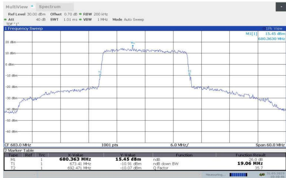
**LTE band 71 , 20MHz Bandwidth,MID,16QAM (-26dBc BW)**
