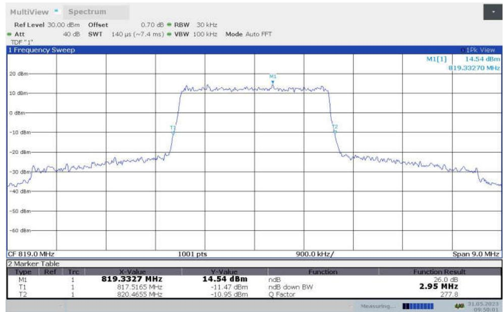
**LTE band 26 , 3MHz Bandwidth,MID,16QAM (-26dBc BW)**
