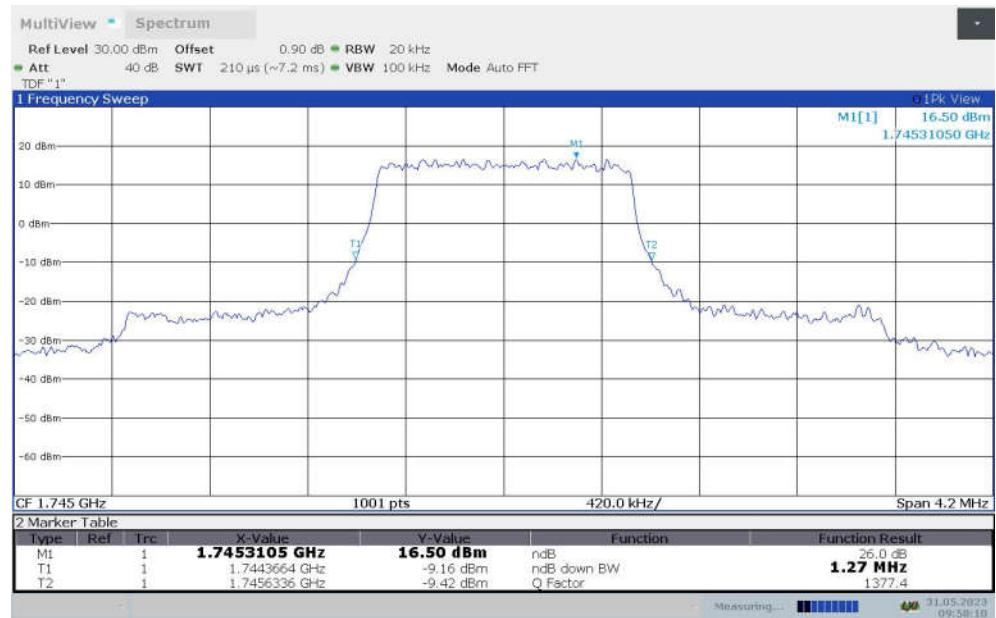
**LTE band 66 , 1.4MHz Bandwidth,MID,16QAM (-26dBc BW)**
