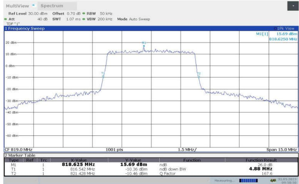
**LTE band 26 (814 MHz-824 MHz),10MHz(-26dBc)**
