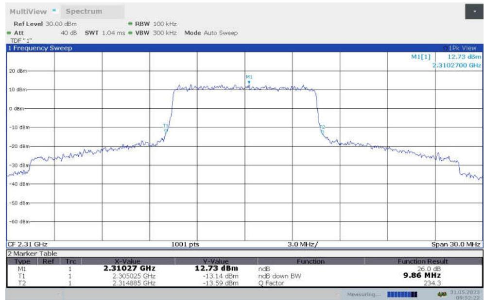
**LTE band 30 , 10MHz Bandwidth,MID,16QAM (-26dBc BW)**
