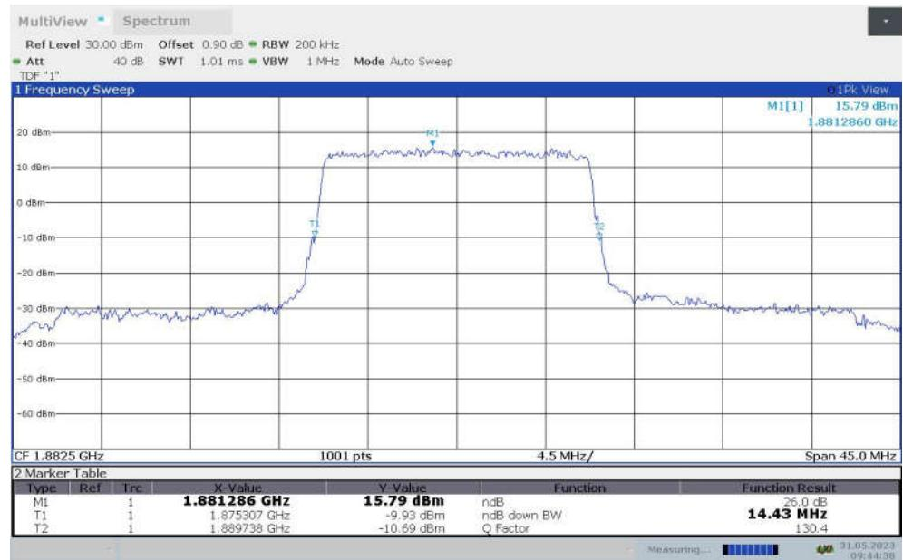
**LTE band 25 , 15MHz Bandwidth,MID,16QAM (-26dBc BW)**
