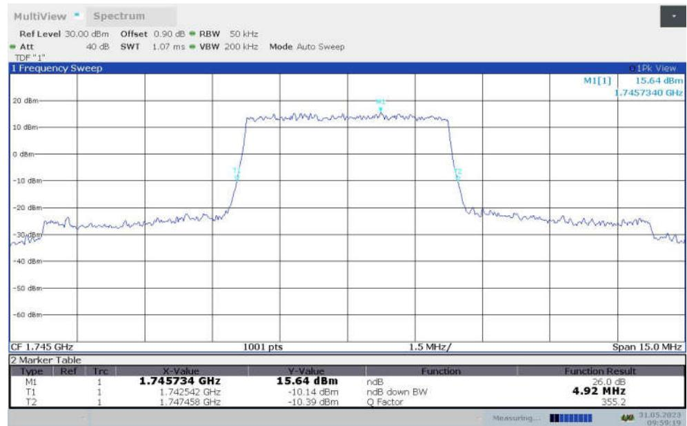
**LTE band 66 , 5MHz Bandwidth,MID,16QAM (-26dBc BW)**
