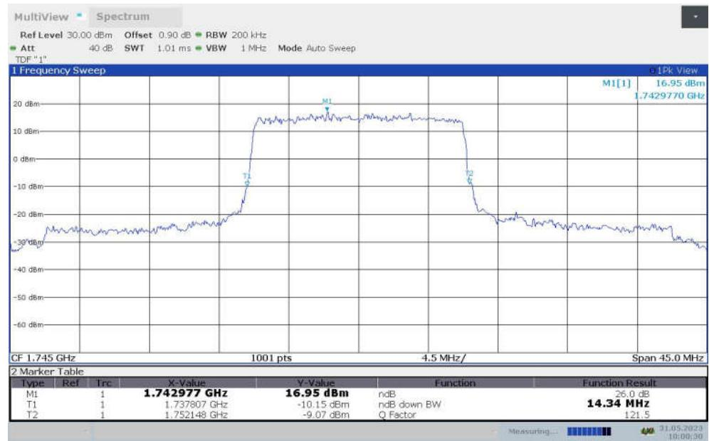
**LTE band 66 , 15MHz Bandwidth,MID,16QAM (-26dBc BW)**
