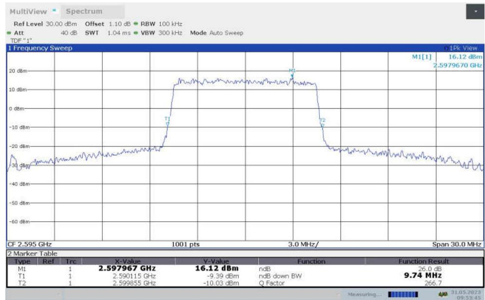
**LTE band 38 , 10MHz Bandwidth,MID,16QAM (-26dBc BW)**
