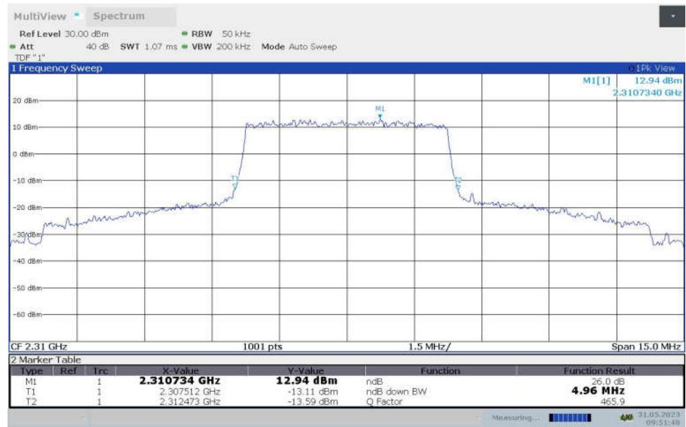
**LTE band 30 , 5MHz Bandwidth,MID,16QAM (-26dBc BW)**
