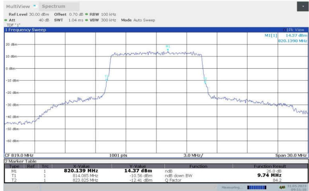
**LTE band 26 , 10MHz Bandwidth,MID,16QAM (-26dBc BW)**
