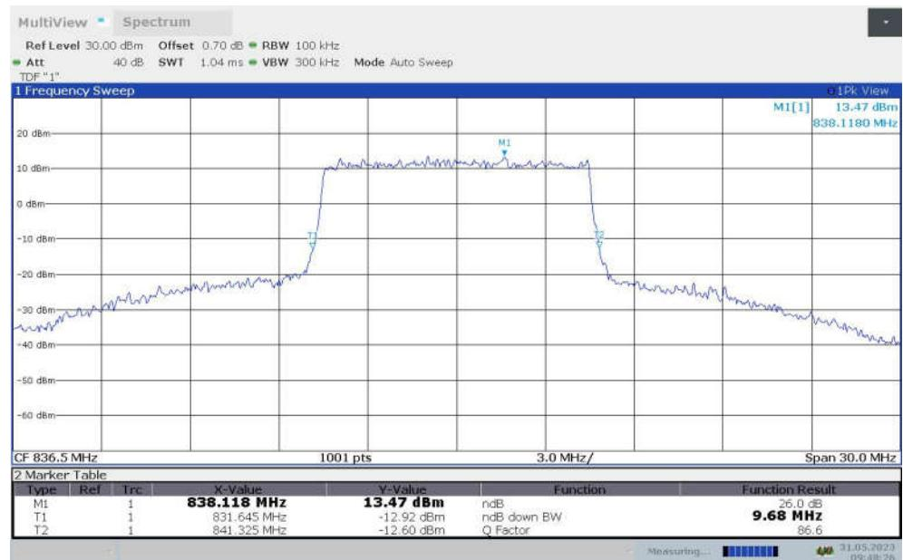
**LTE band 26 (824 MHz-849 MHz),15MHz(-26dBc)**
