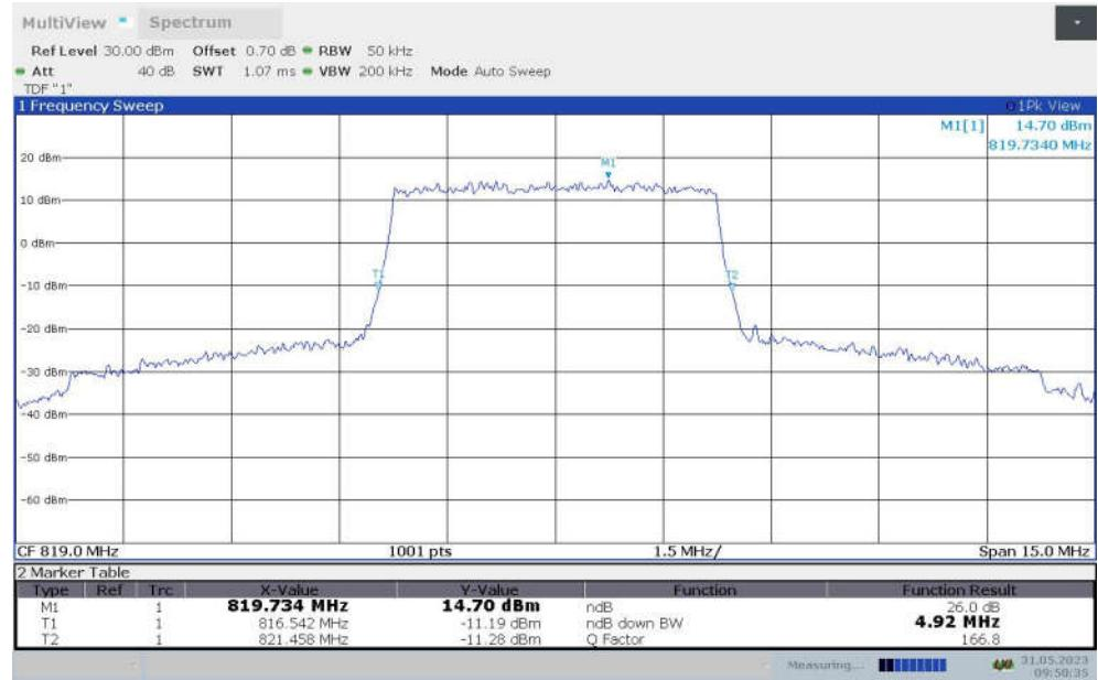
**LTE band 26 , 5MHz Bandwidth,MID,16QAM (-26dBc BW)**
