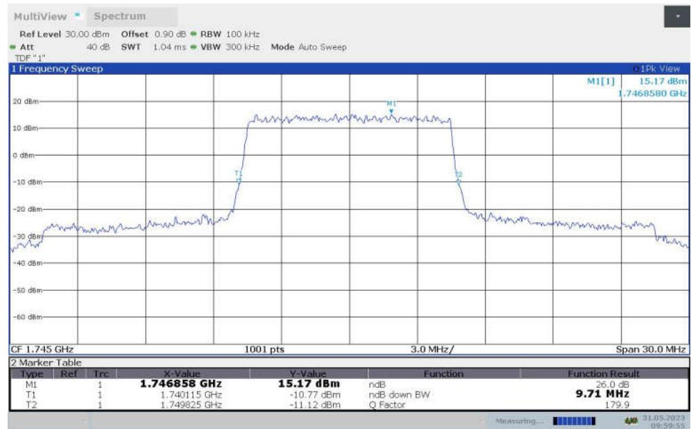
**LTE band 66 , 10MHz Bandwidth,MID,16QAM (-26dBc BW)**
