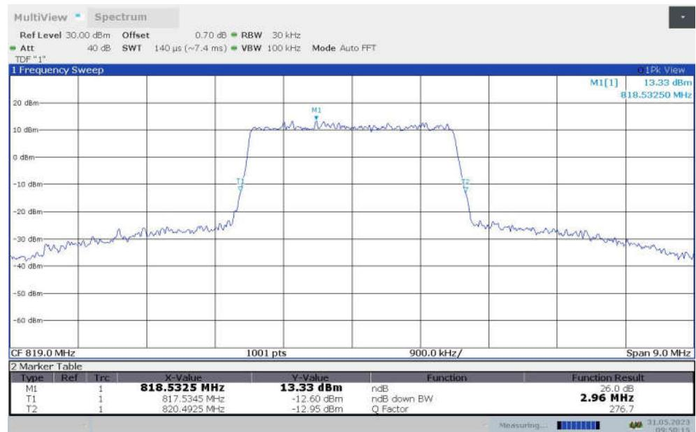
**LTE band 26 (814 MHz-824 MHz),5MHz(-26dBc)**
