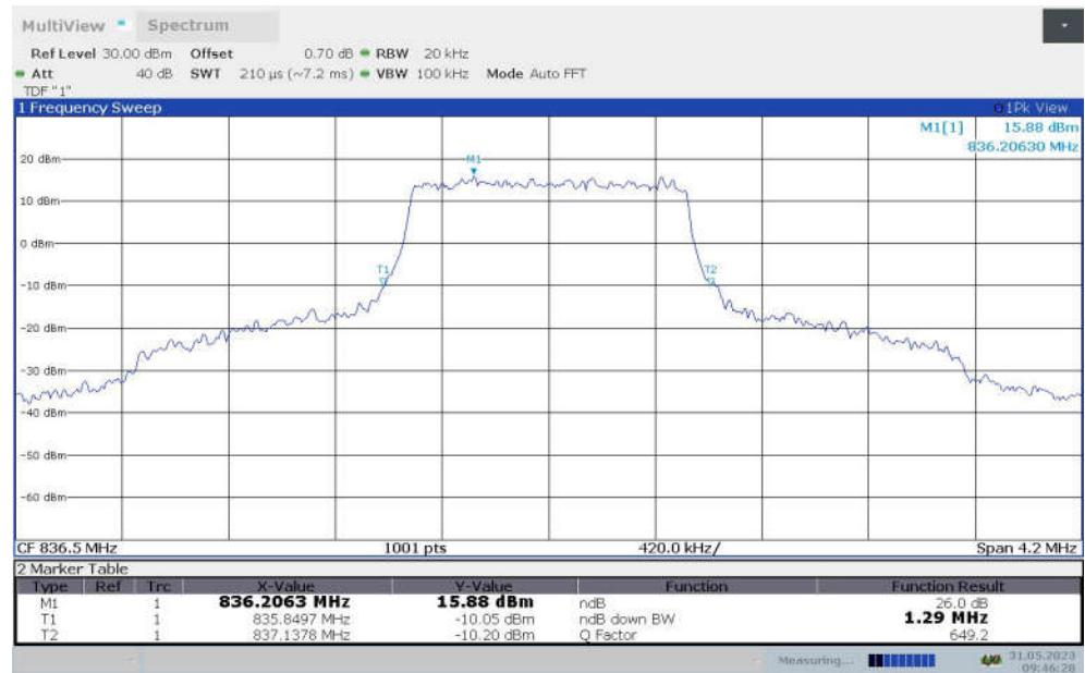
**LTE band 26 , 1.4MHz Bandwidth,MID,16QAM (-26dBc BW)**
