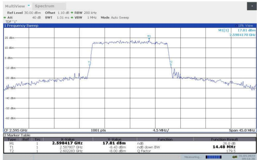
**LTE band 38 , 15MHz Bandwidth,MID,16QAM (-26dBc BW)**
