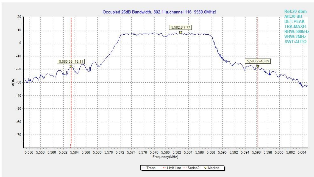
Fig. 8 Occupied 26dB Bandwidth (802.11a, 5580MHz)
