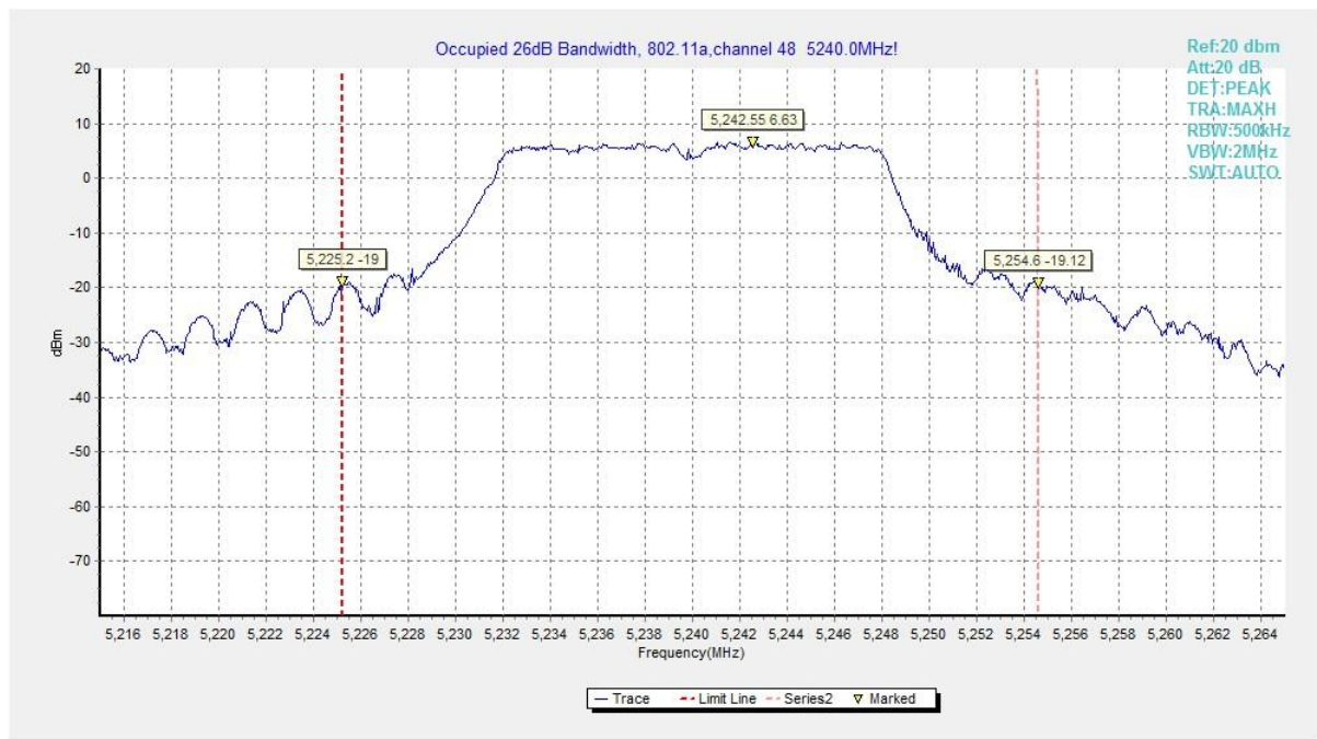
Fig. 3 Occupied 26dB Bandwidth (802.11a, 5240MHz)
