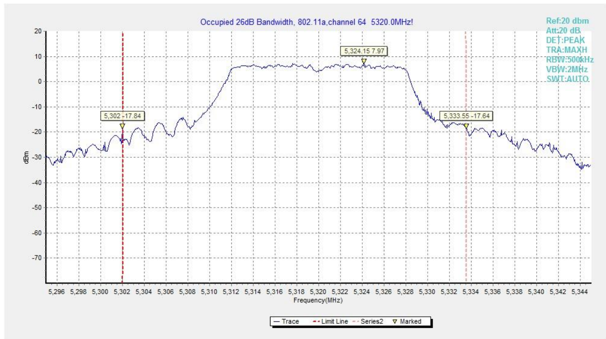
Fig. 6 Occupied 26dB Bandwidth (802.11a, 5320MHz)
