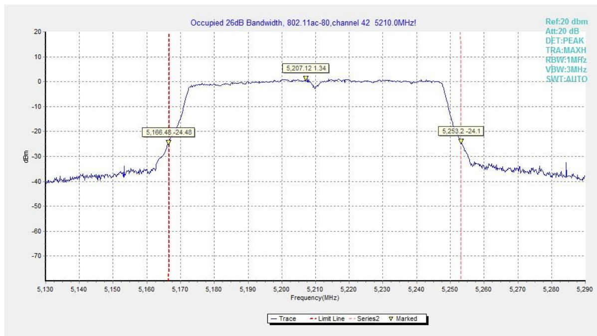
Fig. 16 Occupied 26dB Bandwidth (802. 11ac-VHT80, 5210MHz)
