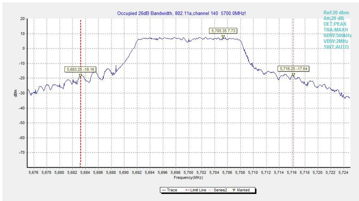
Fig. 9 Occupied 26dB Bandwidth (802.11a, 5700MHz)
