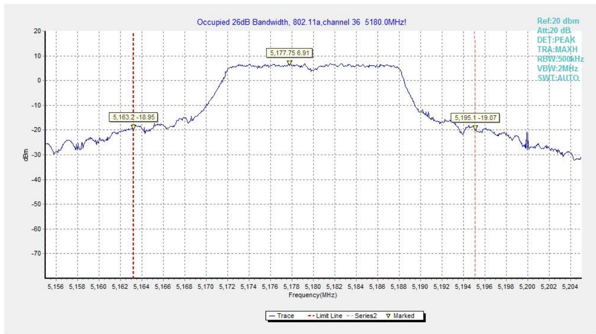
Fig. 1 Occupied 26dB Bandwidth (802.11a, 5180MHz)
