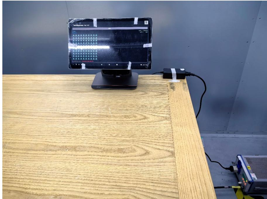
Description: Back view of Conducted Emissions (150kHz-30MHz)
