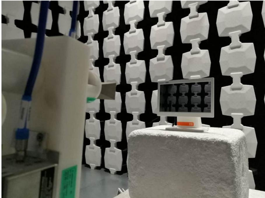
Description: Radiated Emission Test Setup (Above 18GHz)
