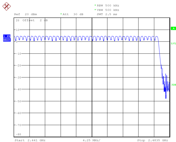
Fig.76 Number of hopping frequency: GFSK, Ch0~39
