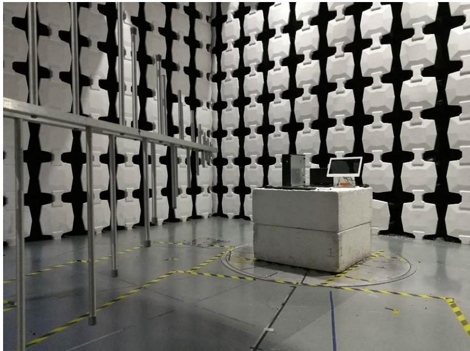
Description: Radiated Emission Test Setup
