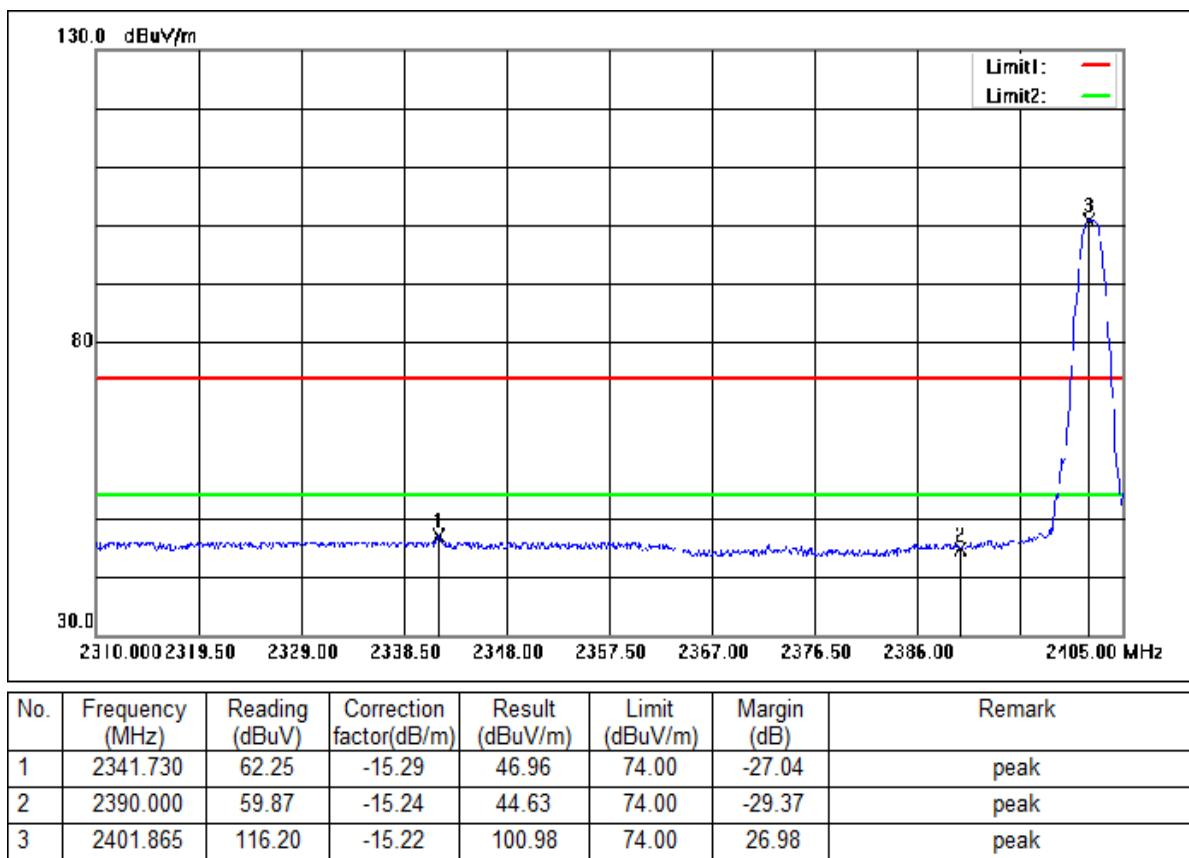
Mode:b; Polarization:Vertical; Modulation:GFSK; ; Channel:Low
