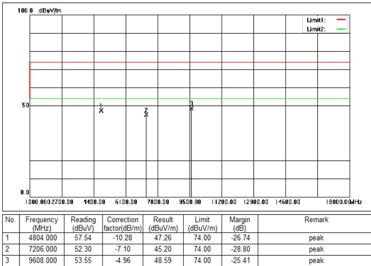
Mode:b; Polarization:Vertical; Modulation:GFSK; ; Channel:Low
