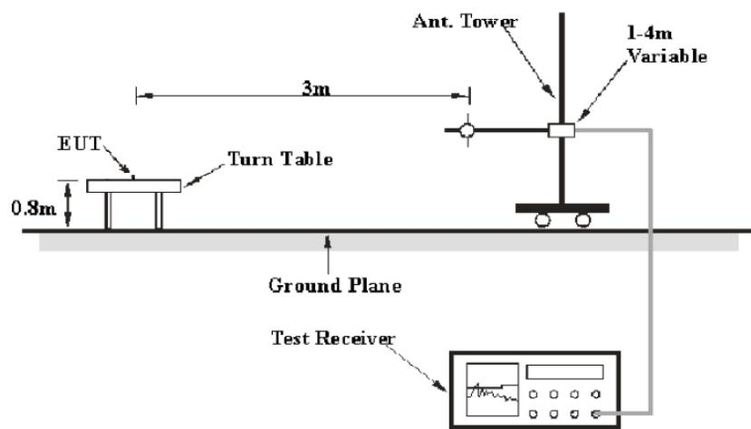
The radiated emission tests were performed in the 3 meters, using the setup accordance with the ANSI C63.10-2013. The specification used was the FCC 15.209 and FCC 15.247 limits.
