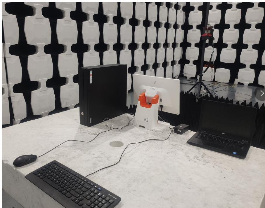
Description: Back view of Radiated Emission Test Setup (Above 1G)
