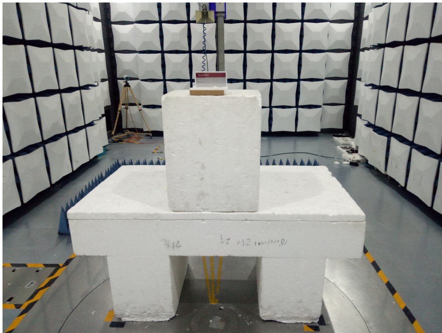
Radiated Emissions View (Above 1GHz)
