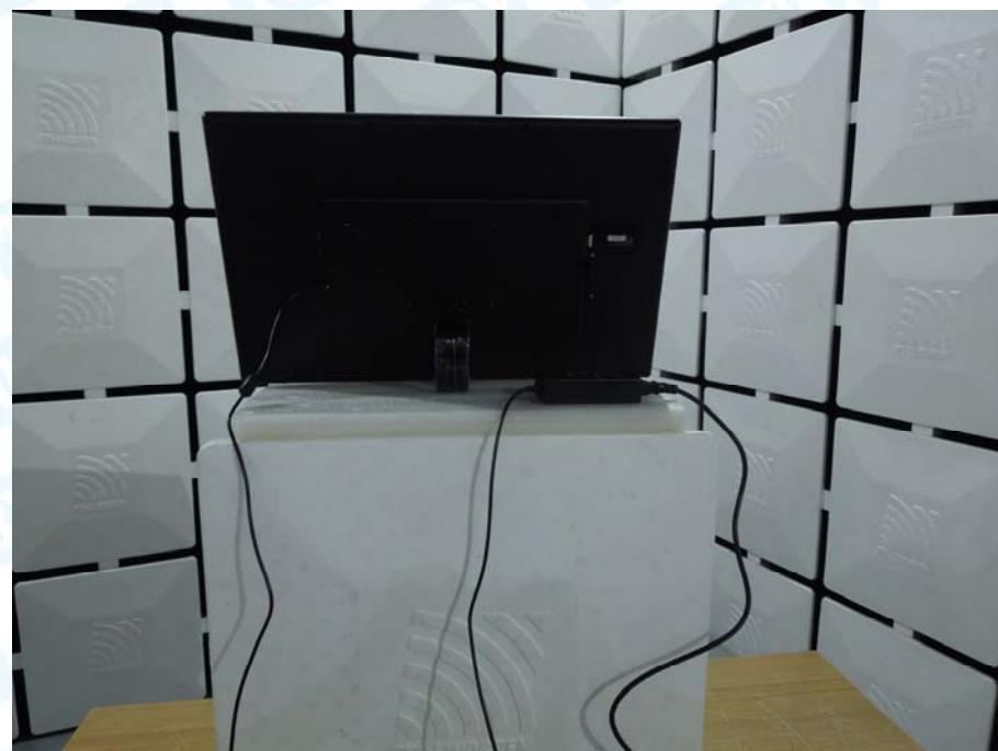
**Photo of Setup for Radiated Emission (Below 1 GHz)**
