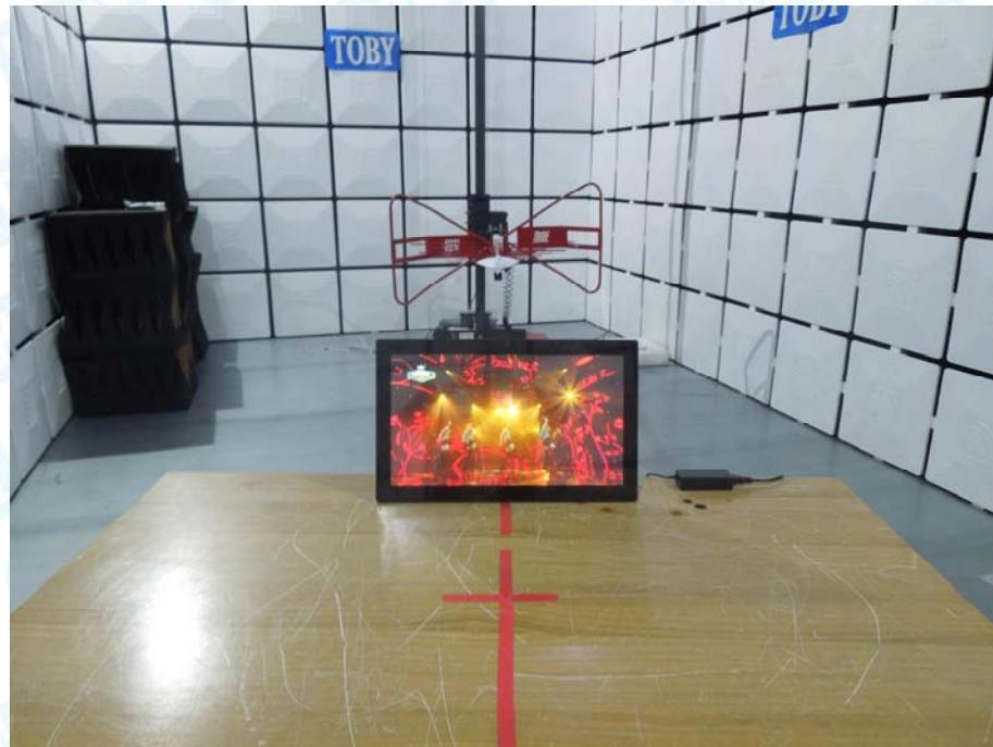
**Photo of Setup for Radiated Emission (Below 1 GHz)**
