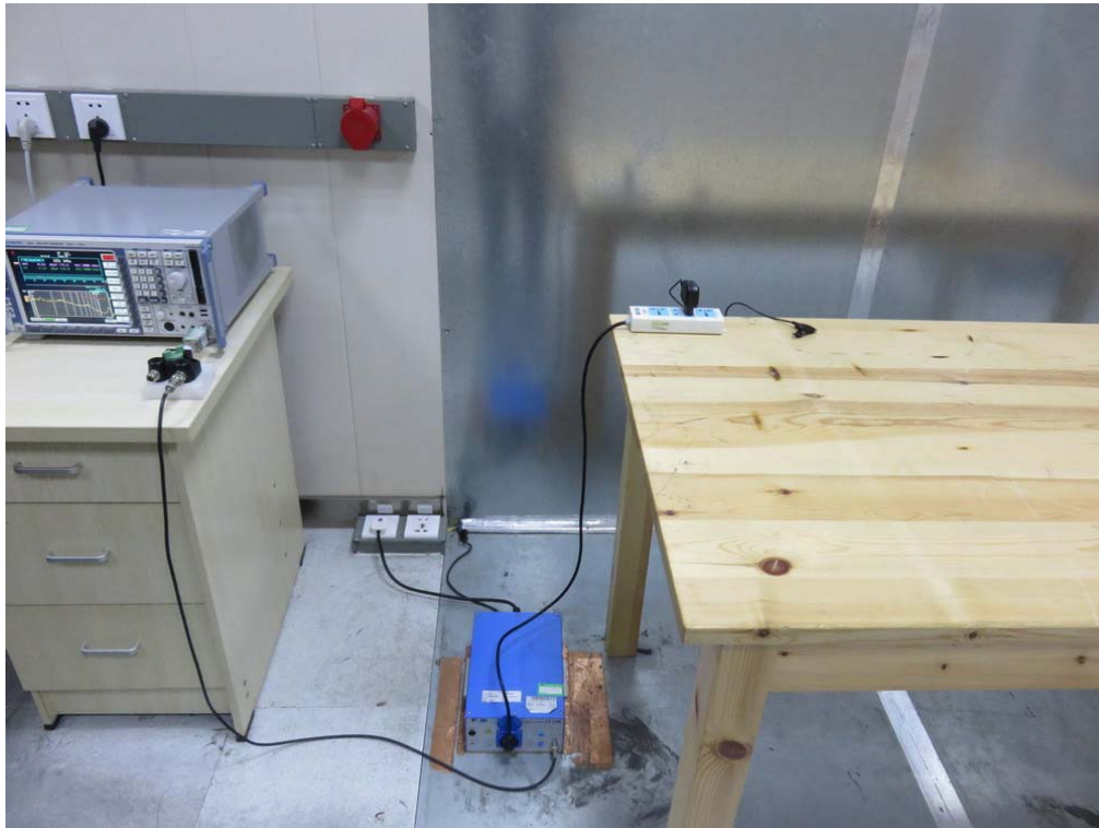
FCC RADIATED EMISSION TEST SETUP
