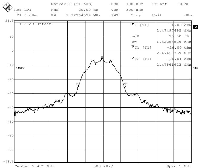
The 20dB bandwidth of emission is contained in the specified frequency band 2400MHz to 2483.5MHz.
