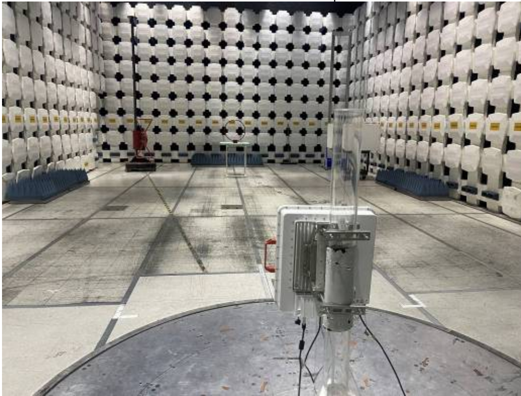
9 kHz-30 MHz Test Setup
