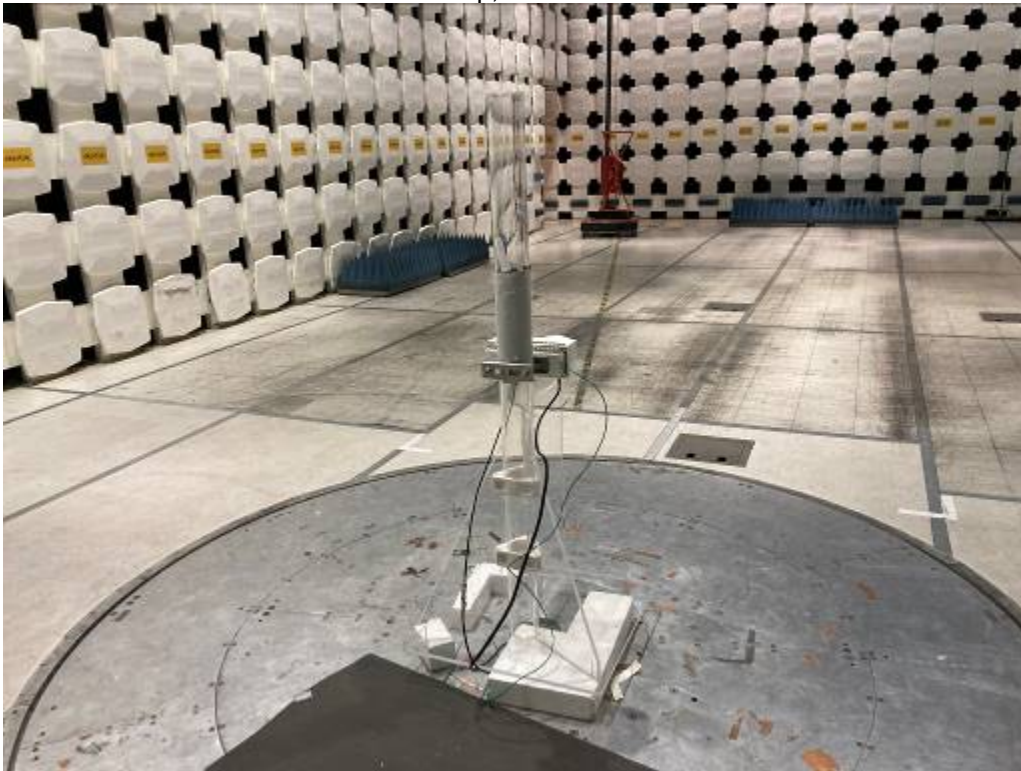
Test Setup, 30-1000 MHz
