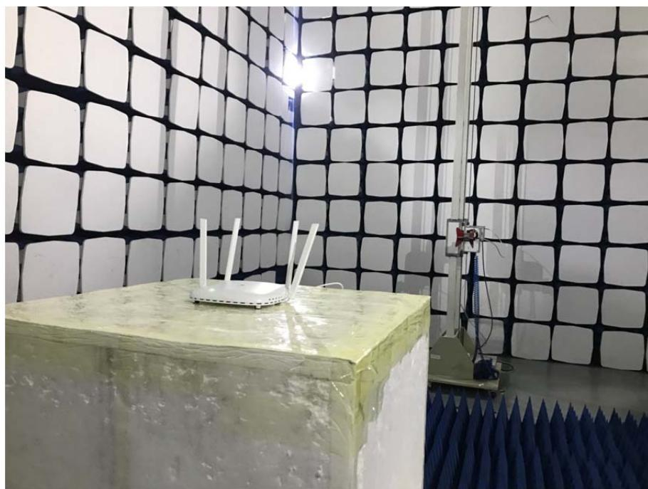
**Radiation Emission Test Setup (Above 18GHz)**
