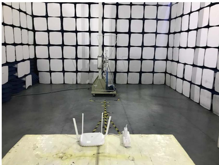
**Radiation Emission Test Setup (1GHz to 18GHz)**
