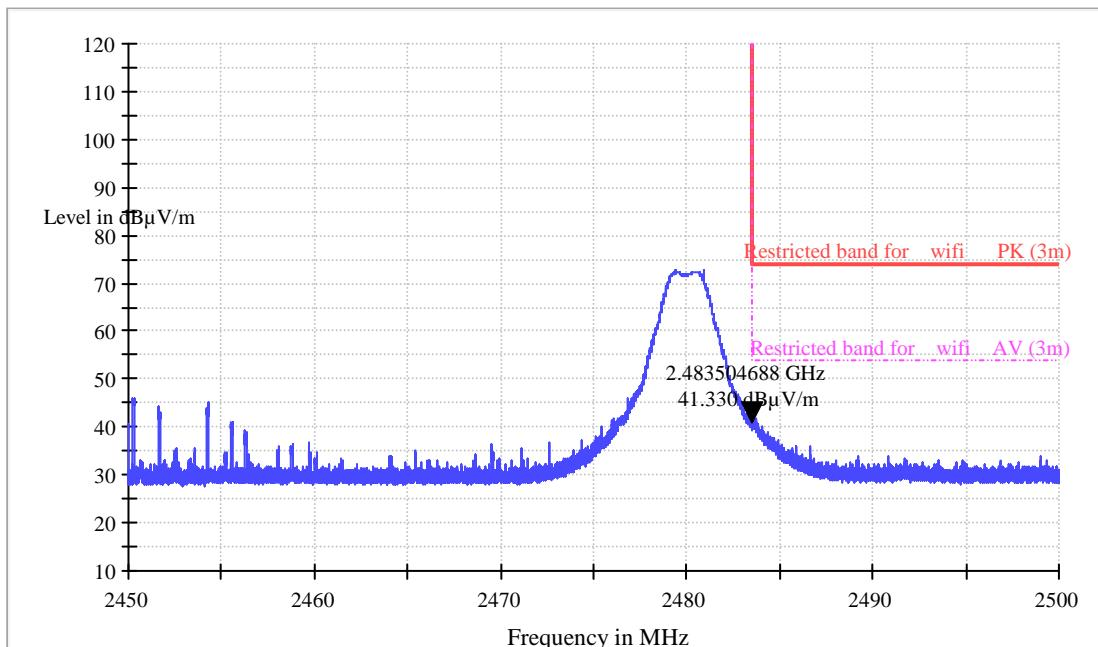
The field strength is calculated by adding the Antenna Factor, Cable Factor & Preamplifier. The basic equation with a sample calculation is as follows:
