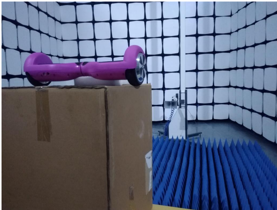
Radiated Emission test view (Above 1GHz)
