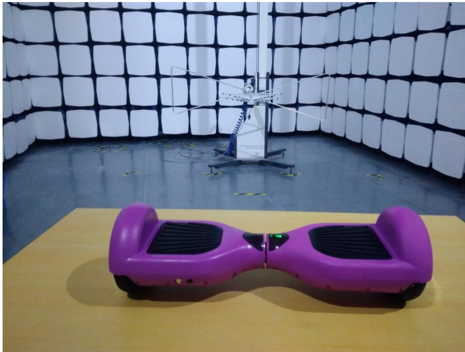
Radiated Emission test view (Below 1GHz)
