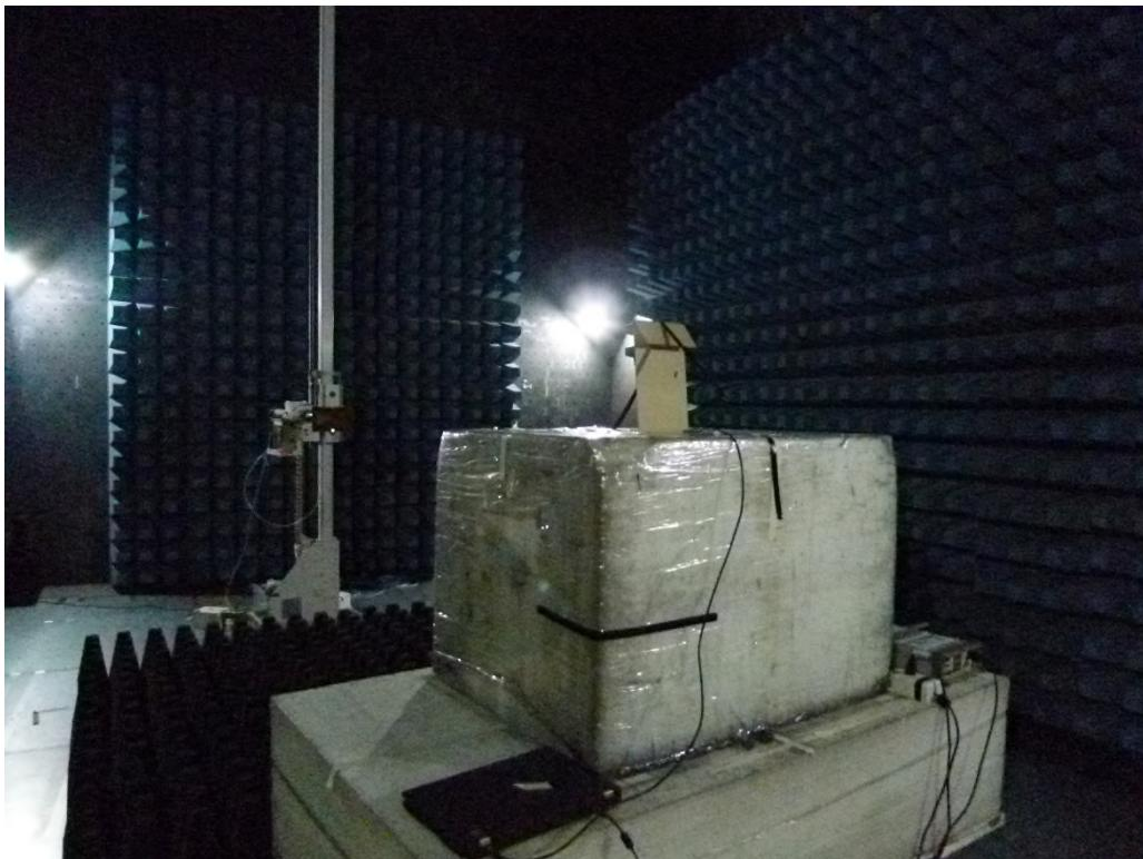
**Radiated Emission Set up Photos (Front View)**
