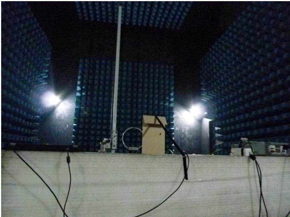
**Radiated Emission Set up Photos (Below 1GHz)**
