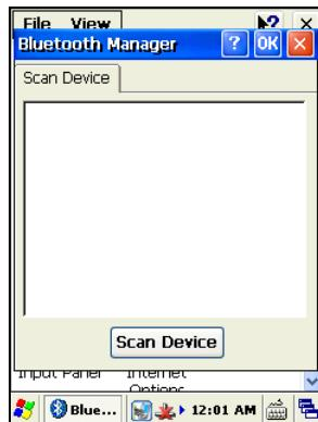
Tap the *Scan Device* button, the handheld begins to scan Bluetooth devices within 10 meters, and show them in the *Scan Device* page, as shown below left. Double tap the device to connect, select the *Trusted* menu item in the appeared menu, as shown below right.
