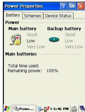
Only when the power part shown in *Main battery* area is as *Good* and 100%, the battery is really fully charged.
