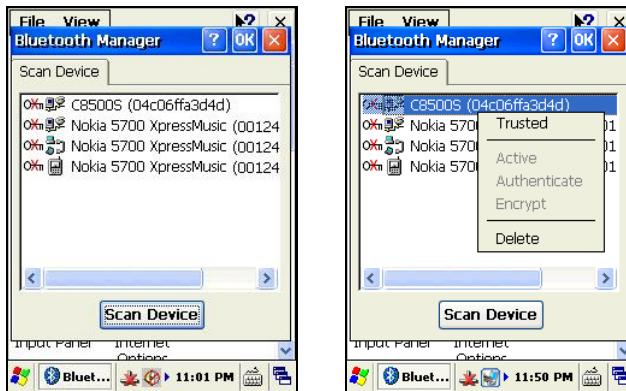
The *Bluetooth Manager* dialog box appeared, as shown below left, tap the *OK* button. Input the matching password (user-defined) in the appeared dialog box, tap the *OK* button, and then wait for inputting the matching password in the other device.
