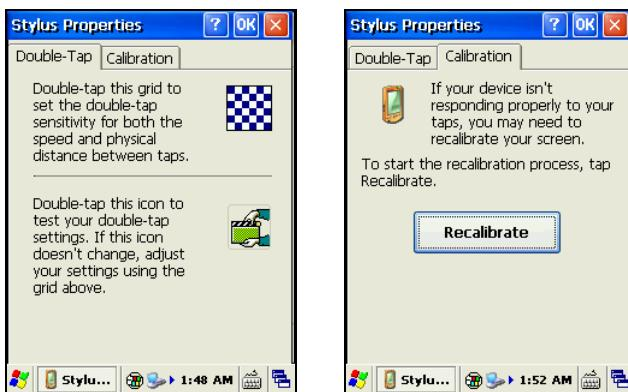
4. Calibrate the touch screen. Tap the *Recalibrate* button to open *Calibration* page. Follow the instructions on the top of the screen to calibrate the touch screen.
