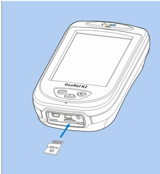
3. You can remove the Micro SD card by lightly pressing the card to make it half pop-out automatically, and then pull it out gently.
