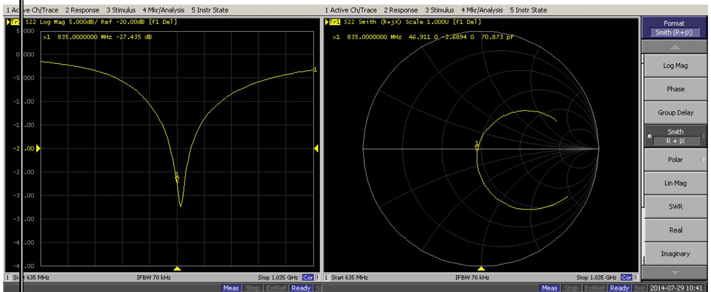
Per IEEE Std 1528-2013, the dipole should have a return loss better than -20dB at the test frequency to reduce uncertainty in the power measurement.
