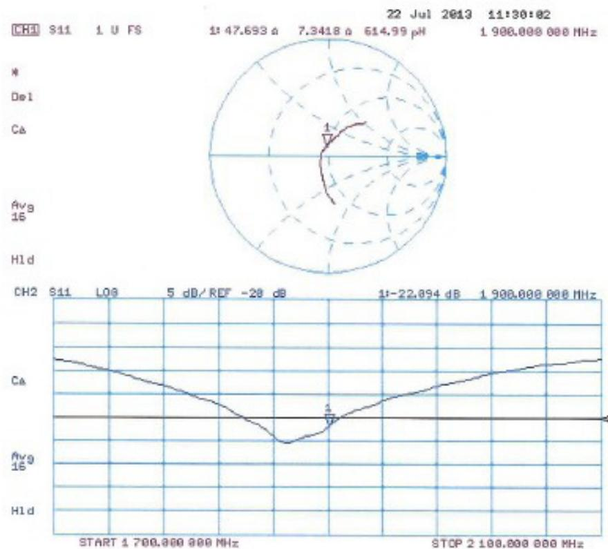
**D1900V2, Serial No.5d136 Extended Dipole Calibrations**
