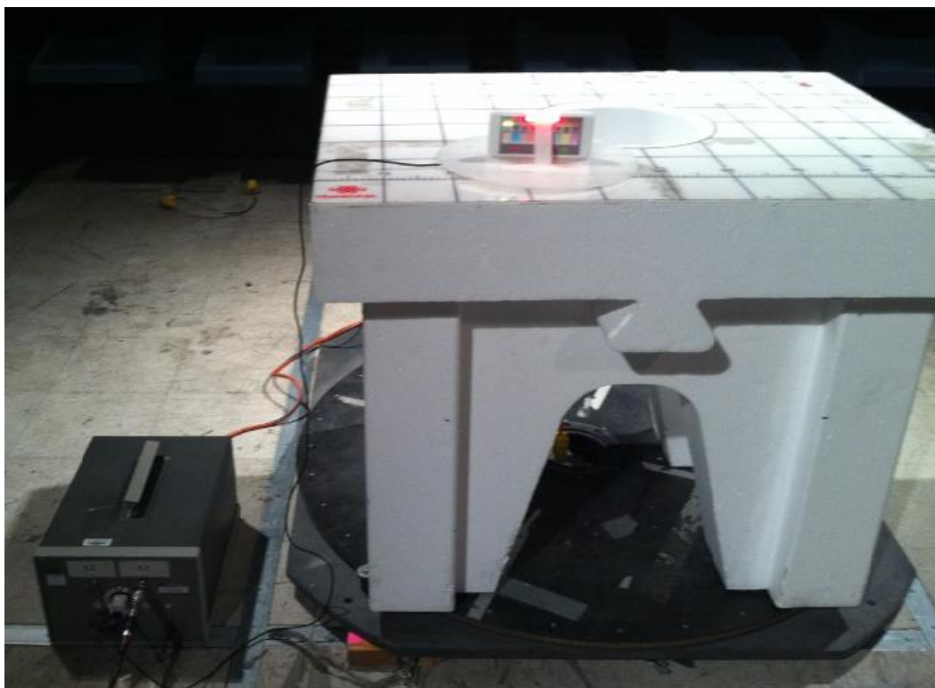
Conducted Emission Test Setup in Semi Anechoic Chamber – 150kHz – 30MHz
