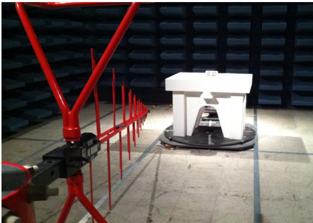
Radiated Emission test setup in Semi Anechoic Chamber – 30MHz - 1GHz
