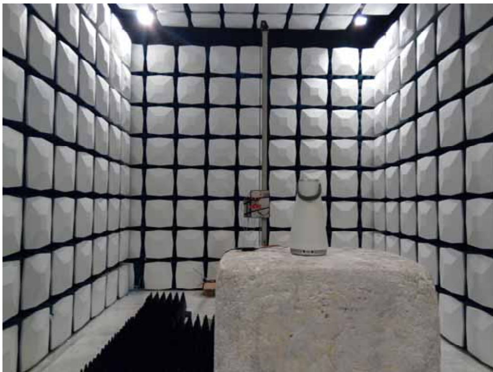
Description: Radiated Emission Test Setup for 1~18GHz
