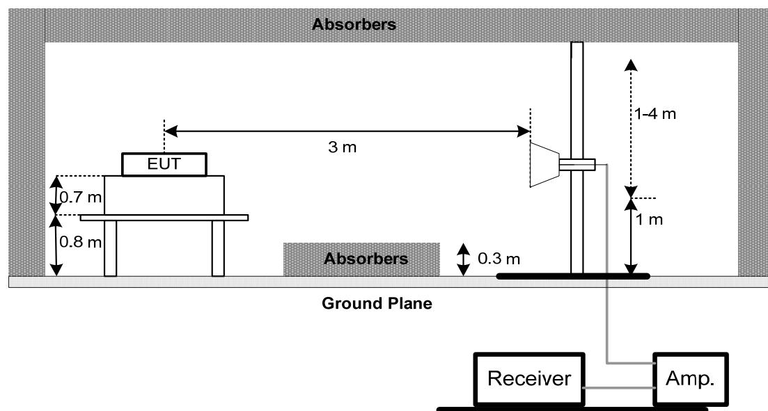
(C) For radiated emissions below 30MHz
