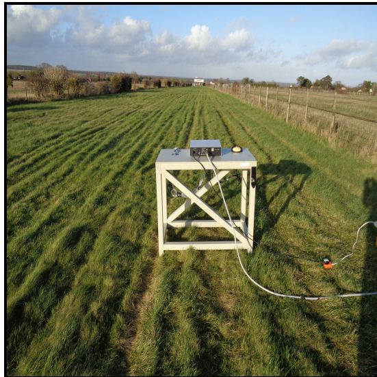
Set up for 300 metre measurements (EUT facing the mag loop antenna)
