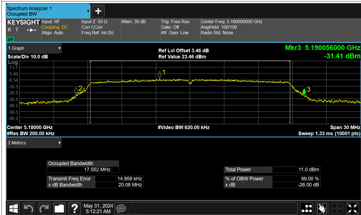
-26dB Bandwidth NVNT n20 5200MHz Ant1
