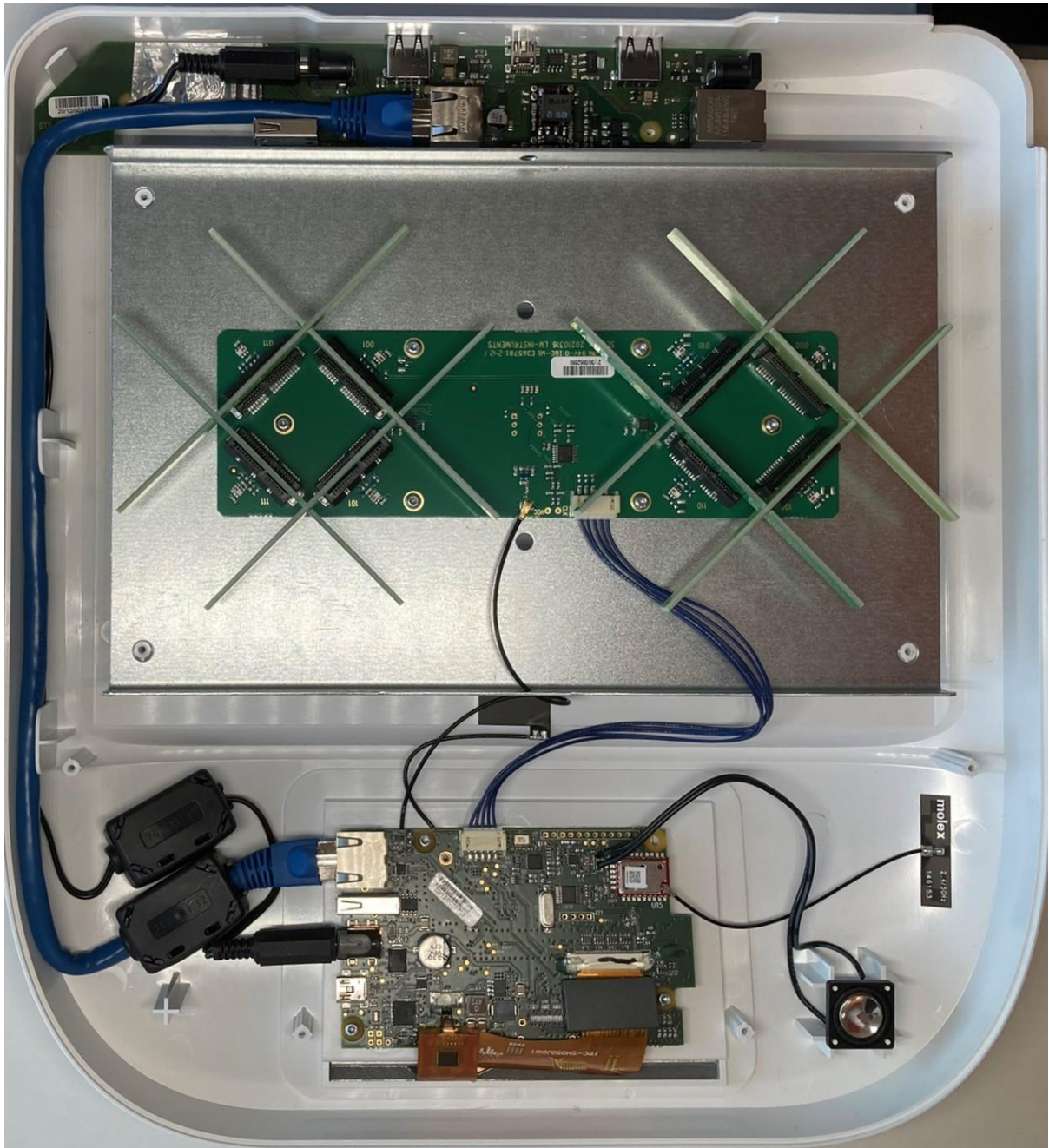
Figure 3 Internal assembly with UHF antenna visible
