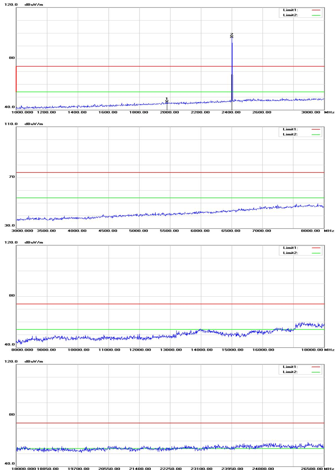
**Above 1 GHz****Operation Mode:** TX / GFSK / DH5 / CH Low**Test Date:** October 15, 2015**Temperature:** 27°C**Tested by:** Jason Lu**Humidity:** 53 % RH**Polarity:** Ver. / Hor.
