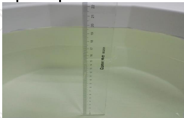
The Body Liquid of 835MHz (15.4cm)
