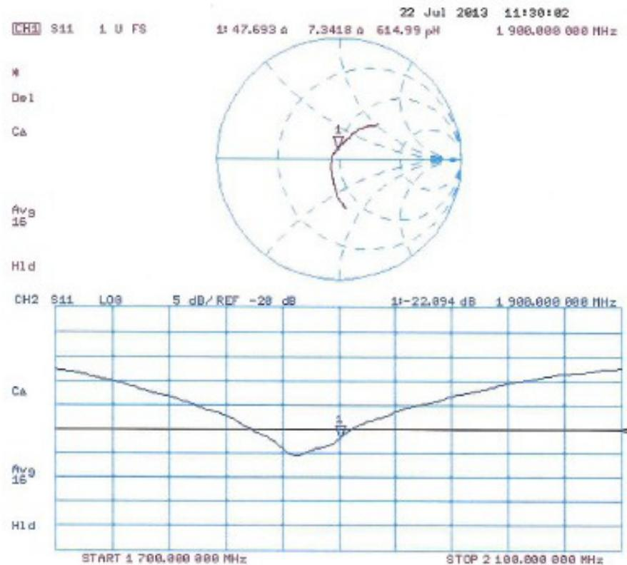
**D1900V2, Serial No.5d136 Extended Dipole Calibrations**
